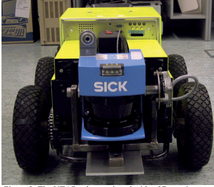
Figure 2: The UTAR robot equipped with a 3D ranging system
