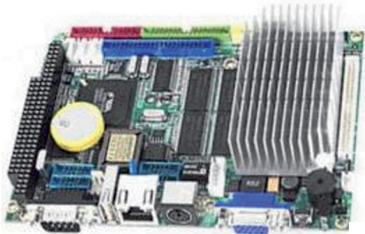
Fig. 5: A PC104 single board computer running on Linux used to produce the terminal device.
