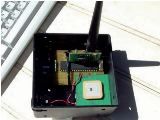
Figure 5. An early prototype pack tag. This tag is equipped with a GPS unit, tri-axial accelerometer, light and temperature sensors.
