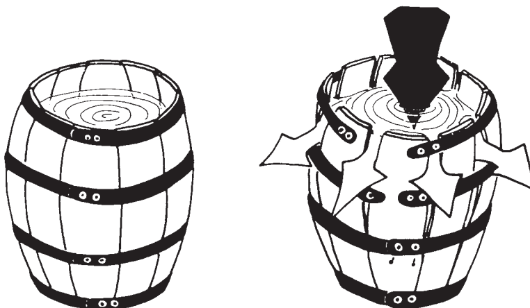
FIGURE 1-7 • Hoop stress. This diagram shows how the load of water in a barrel is resisted by the hoops around the barrel. When too great a load is applied, the hoops will break. The annulus functions in a manner similar to that of the hoops around a water barrel.
