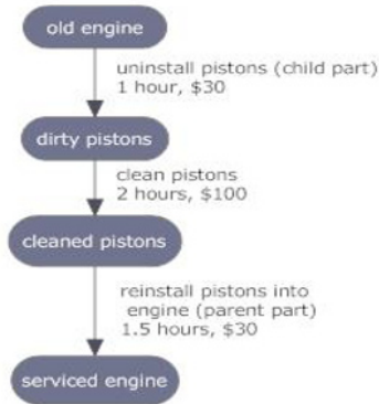
Figure 3: Servicing Pistons. The acts of Labour are the arrows between the ovals, which represent “states” of the system.
