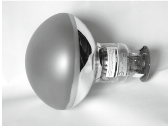
Fig. 9.12 The 9357FLA Electron Tubes photomultiplier. The glass window has been coated with a wavelength shifter in this particular device. Printed from [15] with permission
