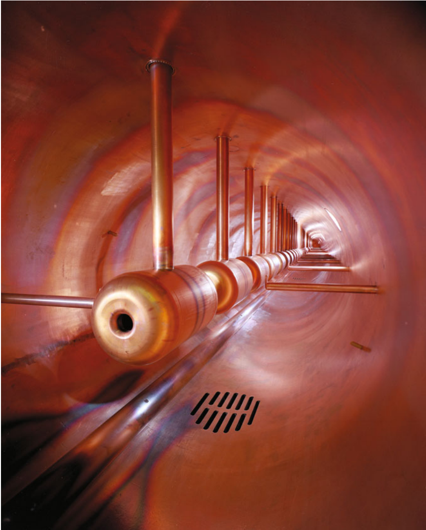
Fig. 5.7 Inside view of the Alvarez-type LINAC at the Fermi National Accelerator Laboratory [7]. Credit Fermilab
