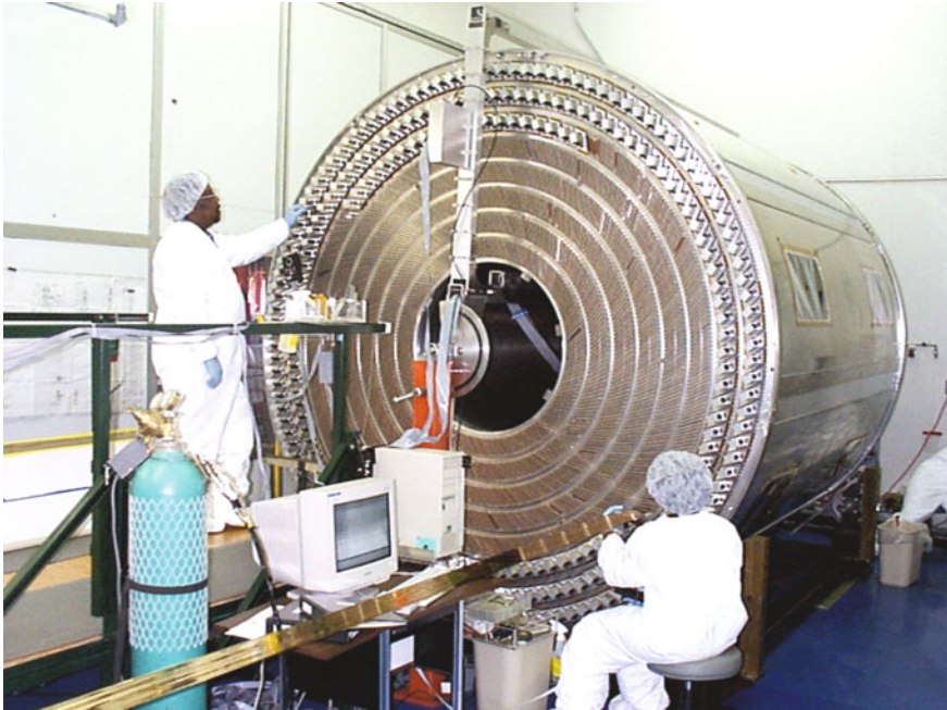
Fig. 7.20 The Central Outer Tracked of the CDF experiment. Reprinted from [13] with permission
