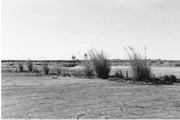
Fig. 8.12. Vetiver and marine couch trials on coal tailings dam. Vetiver grass was one of the only two survivors on this coal tailings dam, which is highly saline, sodic, and high in heavy metals. Vetiver biomass was about ten times greater than marine couch.
