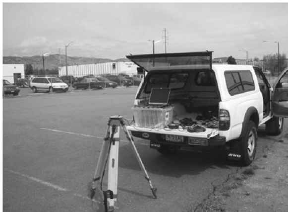
Fig. 7 Collecting data in the field with a Pharos receiver attached to a laptop computer
