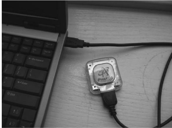
Fig. 6 A photograph of a Pharos single frequency GPS receiver attached to a notebook computer
