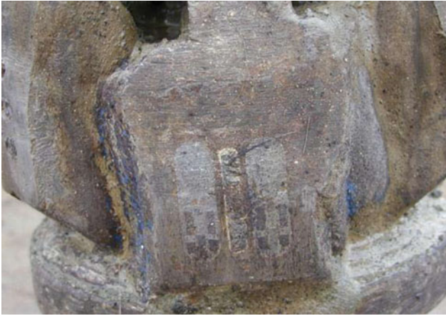
Fig. 7.10 Wearing on gauge of the reaming bit
