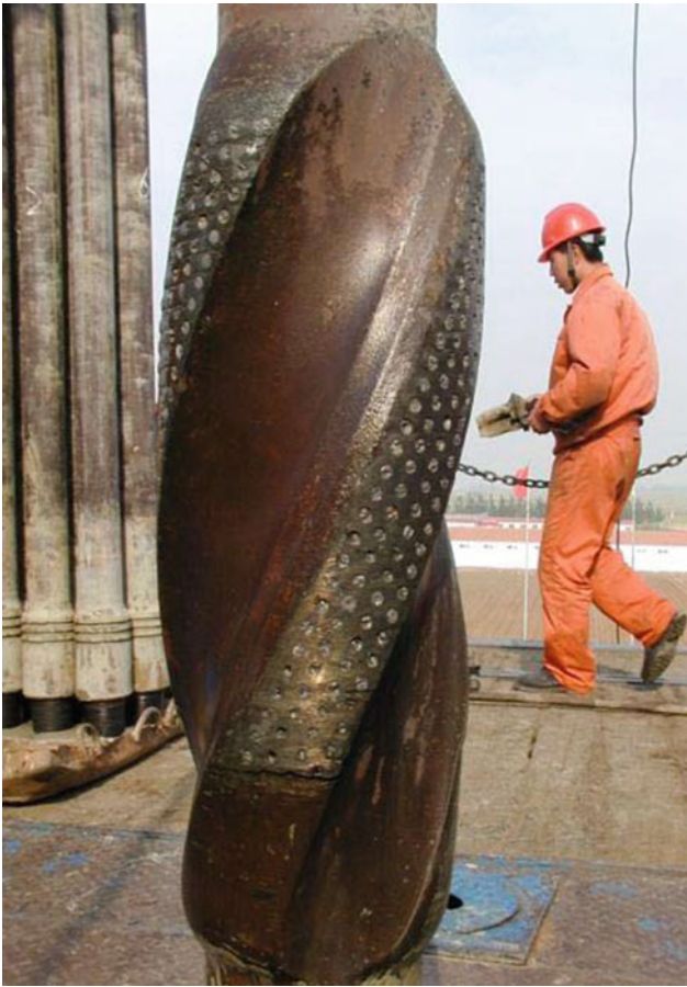
Fig. 7.12 Stabilizer used in reaming drilling
