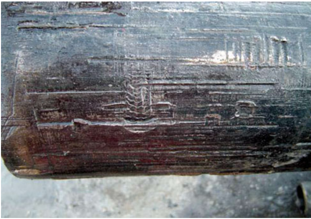
Fig. 5.31 Outer tube damaged by hydraulic pneumatic wrench
