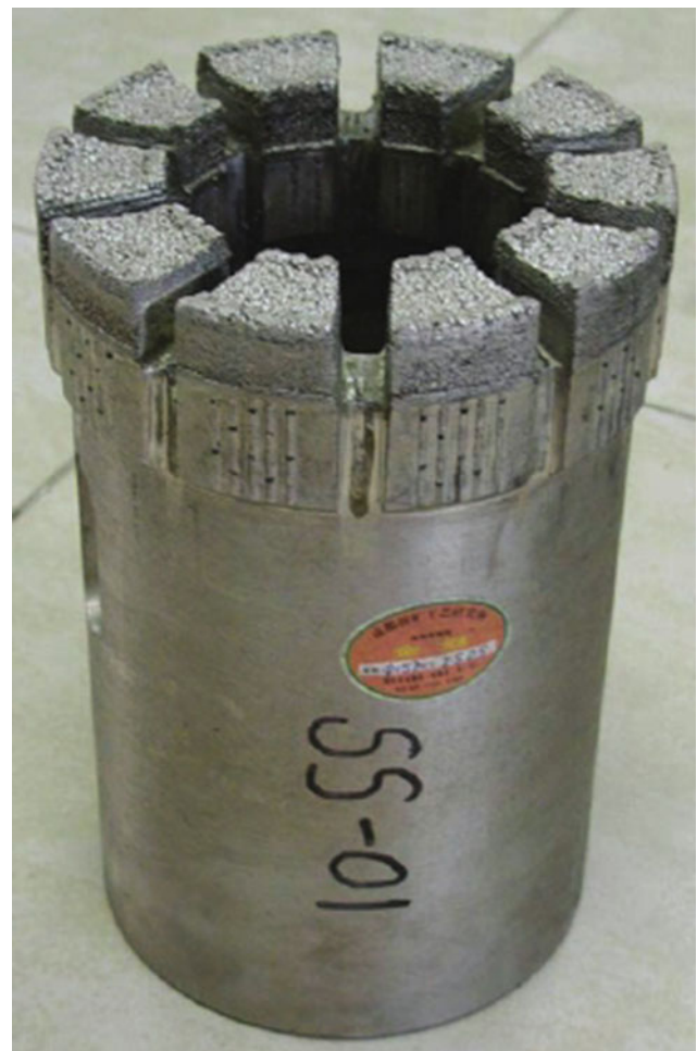
Fig. 6.29 Electro-plated diamond drill bit produced by twice forming
