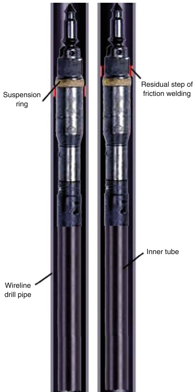
Fig. 5.3 Failure of lowering in and fishing inner tube assembly
