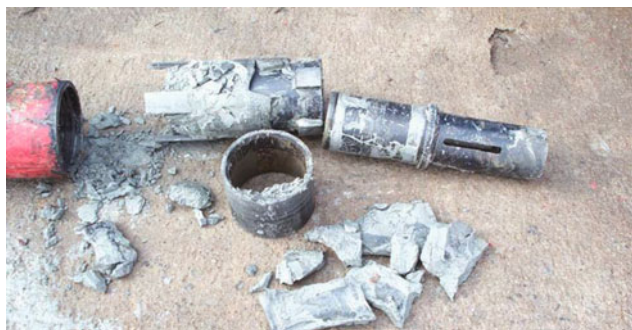
Fig. 5.23 Mud cake in hydro-hammer
