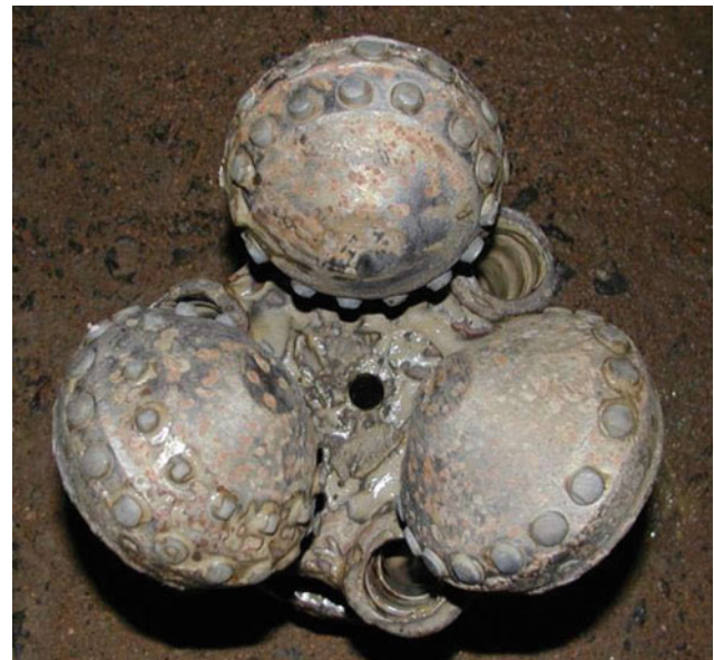
Fig. 7.21 Seriously worn pilot body in MH-2K-21 roundtrip
