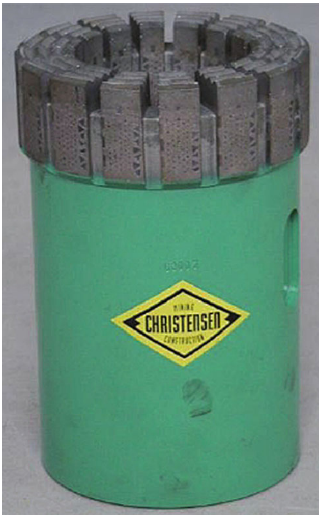
Fig. 6.38 An impregnated drill bit by hot pressing from Germany
