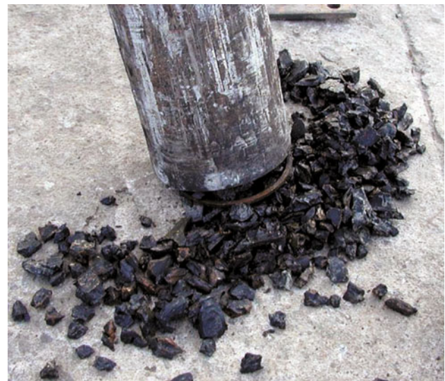
Fig. 5.30 Rubber chips entered into hydro-hammer after PDM degummed
