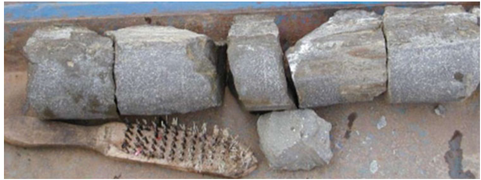
Fig. 8.35 The cement plug samples recovered near the side-tracking point
