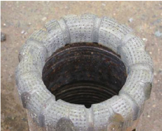
Fig. 6.35 A worn surface set drill bit produced by Chuanke Co. Ltd.
