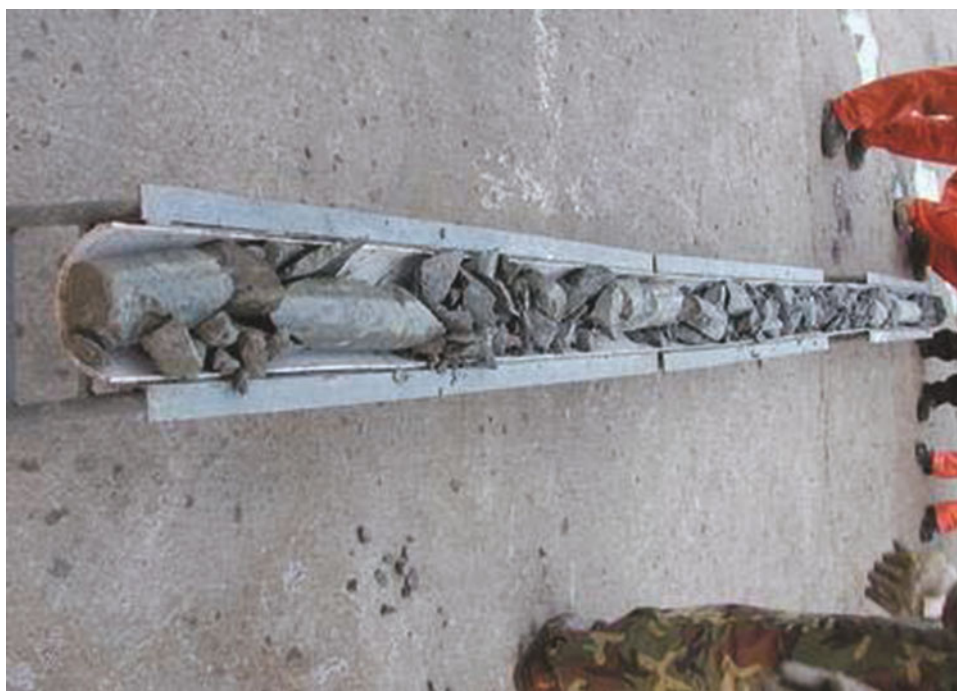
Fig. 5.37 Broken core taken by KZ-1 drilling tool
