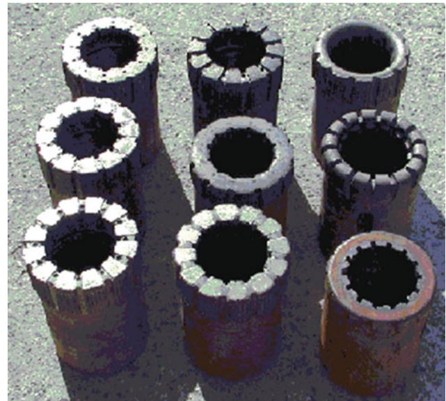
Fig. 6.17 Drill bit wear in top drive core drilling
