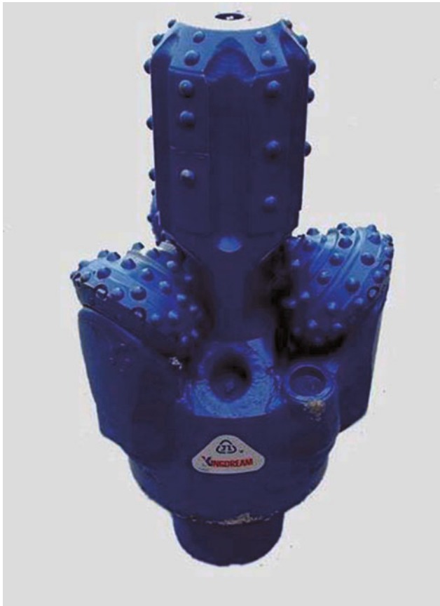
Fig. 7.2 KHAT series of rock bit developed by Kingdream
