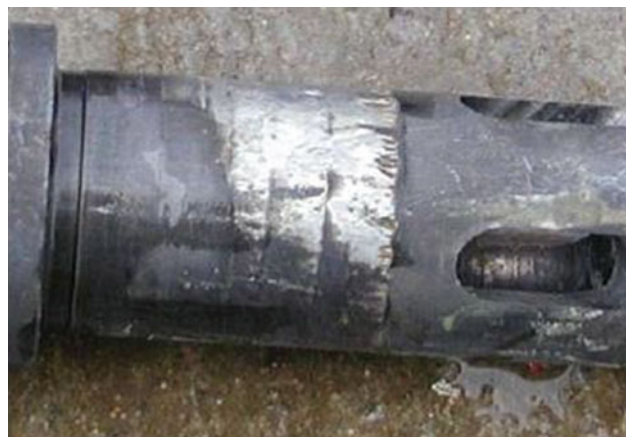
Fig. 5.24 Sealing surface of upper valve was eroded
