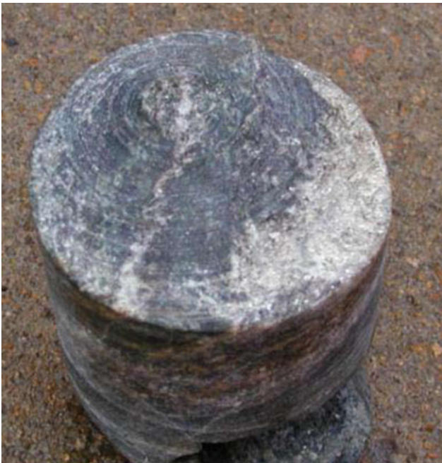
Fig. 8.19 The core recovered at the end point of side-tracking drilling
