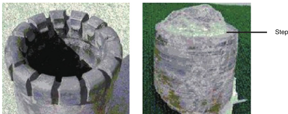
Fig. 6.18 Inner step on the drill bit and the inclined worn core
