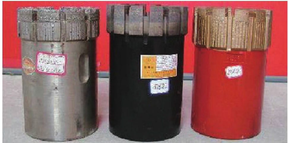
Fig. 6.4 Impregnated diamond core bits. Left Electro-plated drill bit by twice forming method, developed by the Institute of Exploration Technologies. Middle Drill bit by sintering process of hot press, developed by Guilin Diamond Co. Right Segment inserted drill bit by twice forming, developed by the Beijing Institute of Exploration Engineering
