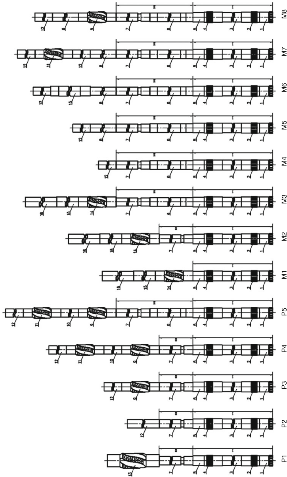
Fig. 8.5 Down hole drilling tool assemblies for CCSD-1 Well. 1 \phi 157 mm coring bit 2, 4 \phi 157 mm reamer 3 \phi 139.7 mm core barrel 5 \phi 146 mm swivel type sub 6 \phi 127 mm hydro-hammer 7 \phi 120 mm PDM 8 \phi 120 mm jar-while-drilling 9, 11 \phi 156 mm stabilizer 10, \phi 120 mm single collar 12 \phi 120 mm collar string 13 \phi 215.9 mm stabilizer 14 SK157 stabilizer 15 SK146 wireline drill collar string 16 SK139.7 wireline drill rod string
