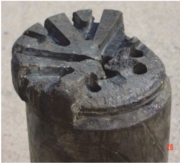
Fig. 8.27 140 mm impregnated drill bit with matrix fell off
