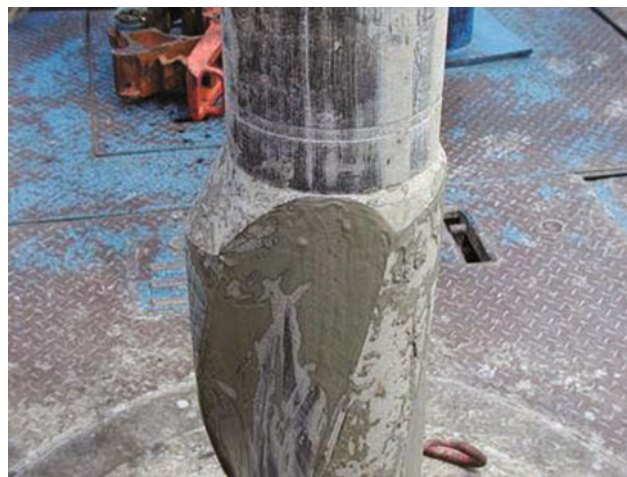
Fig. 8.7 Serious one-side wearing of the stabilizer when drill string turning
