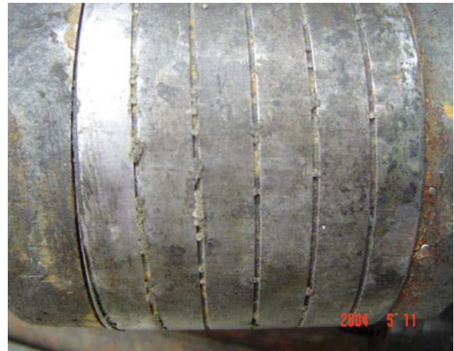
Fig. 5.29 Plastic balls in the clearance of piston
