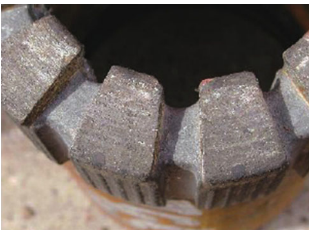
Fig. 6.3 Diamond exposure under the percussion of hydro-hammer
