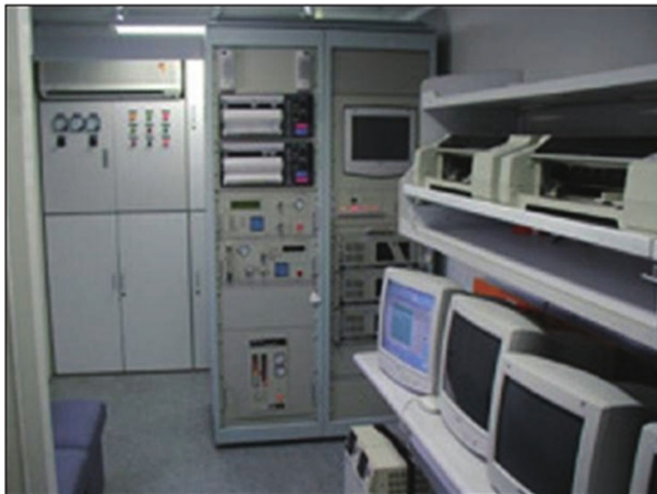
Fig. 11.1 The internal units of SK-2000FC/C comprehensive logging instrument developed by Shanghai Shenkai company
