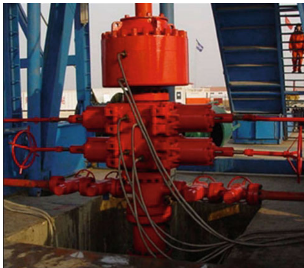
Fig. 3.18 FH35-35 double-ram BOP
