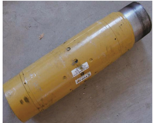
Fig. 10.16 193.7 mm stage collar
