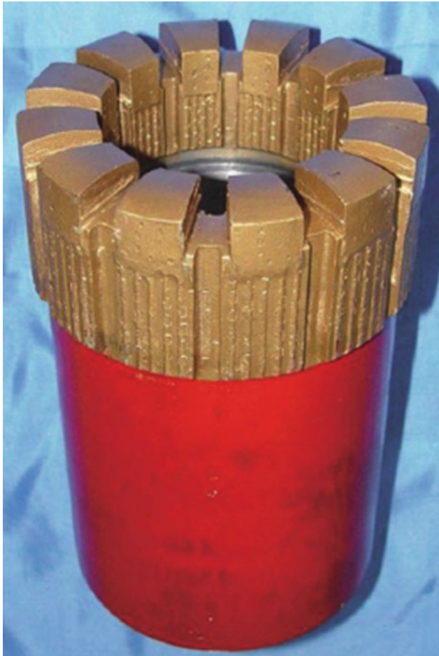
Fig. 6.23 Diamond segment inserted core drill bit produced by twice forming
