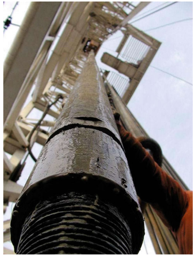
Fig. 5.22 The hydro-hammer worked for five continuous round trips
