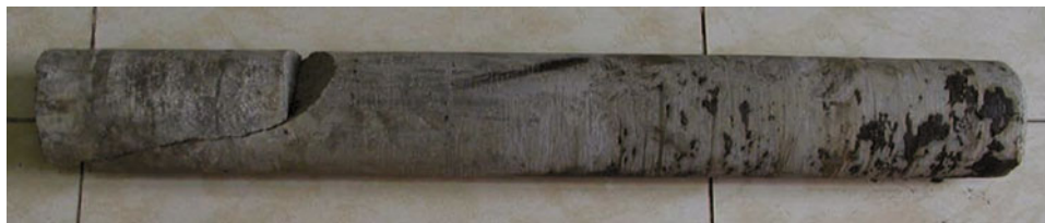
Fig. 8.12 The cement plug sample in the side-tracking drilling point
