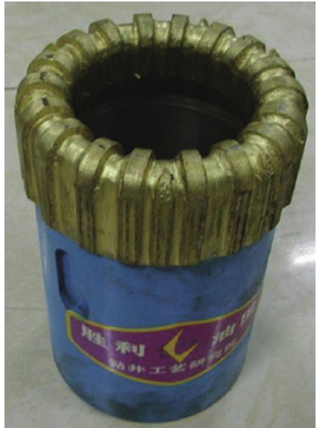
Fig. 6.37 An impregnated drill bit by hot pressing from the Tool Institute, Drilling Research Academy of Shengli Oil Field
