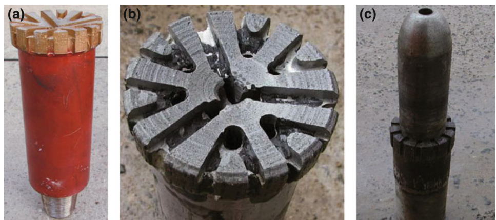
Fig. 8.15 Drill bits for small diameter side-tracking drilling. a φ 140 mm impregnated bit. b φ 140 mm impregnated bit after side-tracking drilling. c φ 157 mm reaming bit with guide
