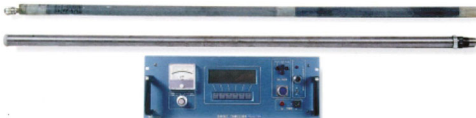
Fig. 11.4 The electromagnetic down-hole drilling parameter acquisition system from Geoservice Company
