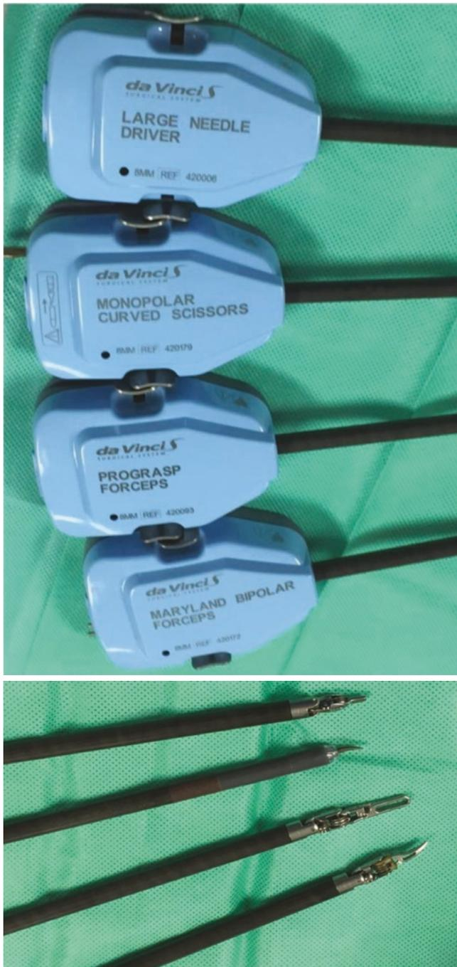
**Fig. 4.11** Examples of some of EndoWrist instruments
