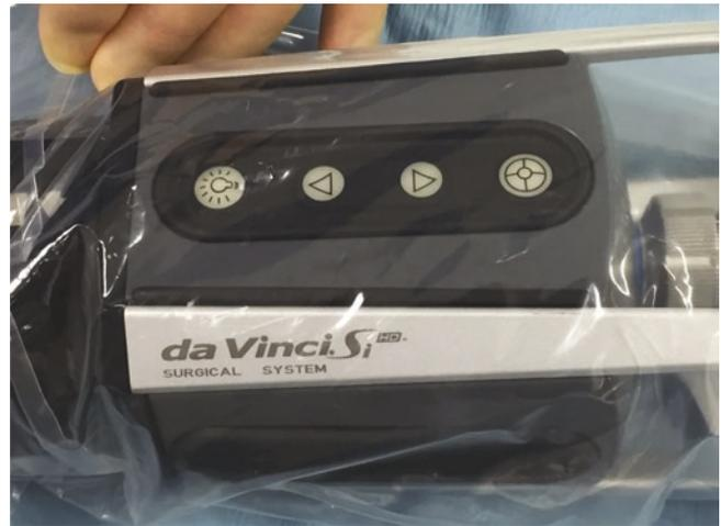
**Fig. 4.9** The HD stereo camera
