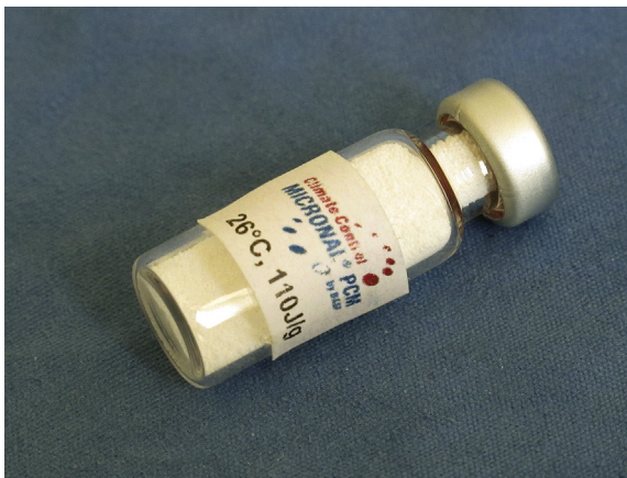
Figure 5.10 BASF Micronal microencapsulated phase-change material. Photo by the author.
