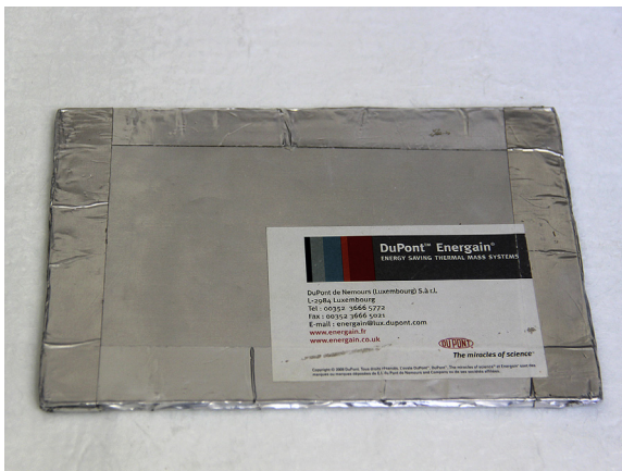
Figure 5.14 DuPont Energain phase-change material panel. Photo by the author.
