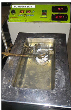
Fig. 2 Schematic representation and actual photograph of an ultrasonic bath
