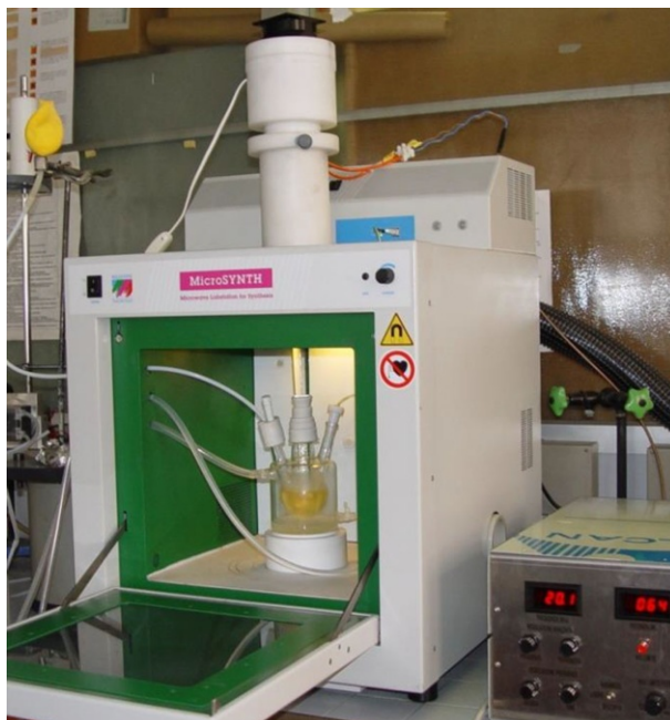
Fig. 10 Transesterification under SMUI (authors' laboratory)
