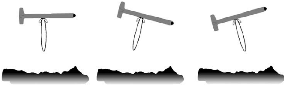
Figure 10.17. Unprocessed pitch of the sonar platform will replicate previous swath lines (pitch < 0) or anticipate future swath lines (pitch > 0).
