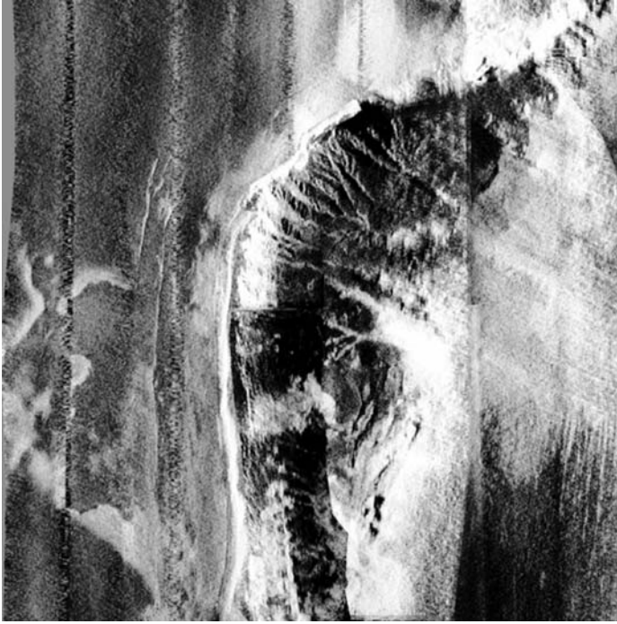
Figure 7.28. GLORIA regional imagery of the Blake Escarpment, on the continental margin east of Florida. The image is 51 km wide and 51 km long, oriented with north at the top. Depths vary abruptly between 2,500 m in the left half of the image and 4,900 m in the right half (courtesy United States Geological Survey).
