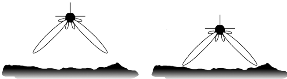
Figure 10.14. When the sonar is at a higher altitude above the bottom the swath width will increase. If the system erroneously records higher altitudes than the real one the image will be compressed across-track. Conversely, if the system records lower altitudes the image will be stretched across-track.
