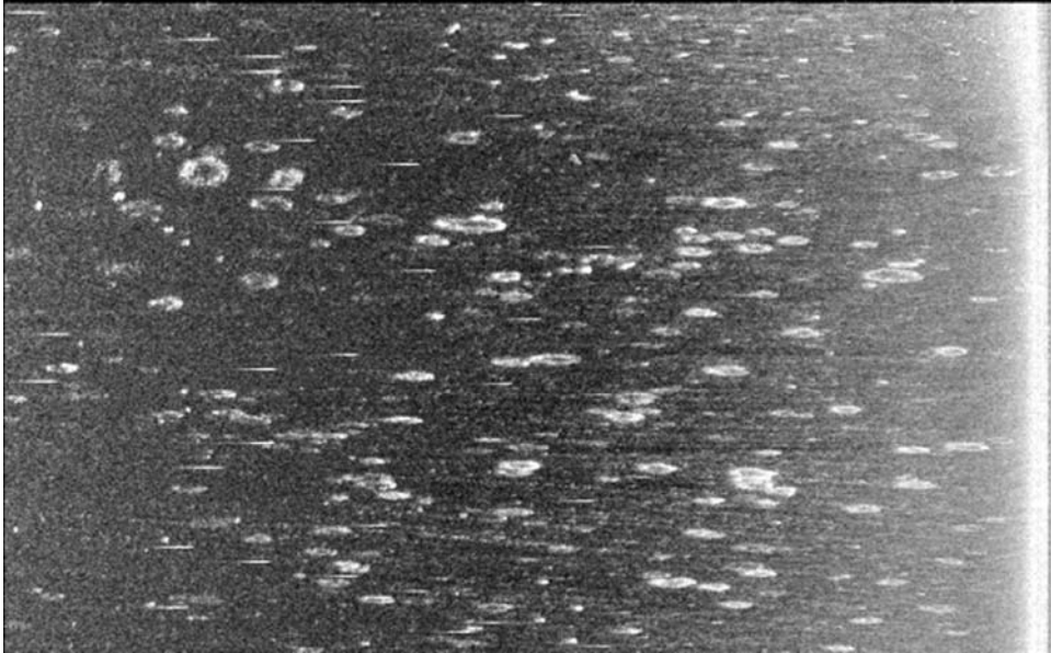
Figure 8.15. High-resolution image of old oyster beds in a shallow lake, acquired with the SwathPlus interferometric, multi-frequency system. The image is 100 m wide and ensonified from the right. Note the across-track distortion of the structures increasing with range, which can be processed using the steps outlined in Chapter 4 (image courtesy SEA Ltd., U.K.).
