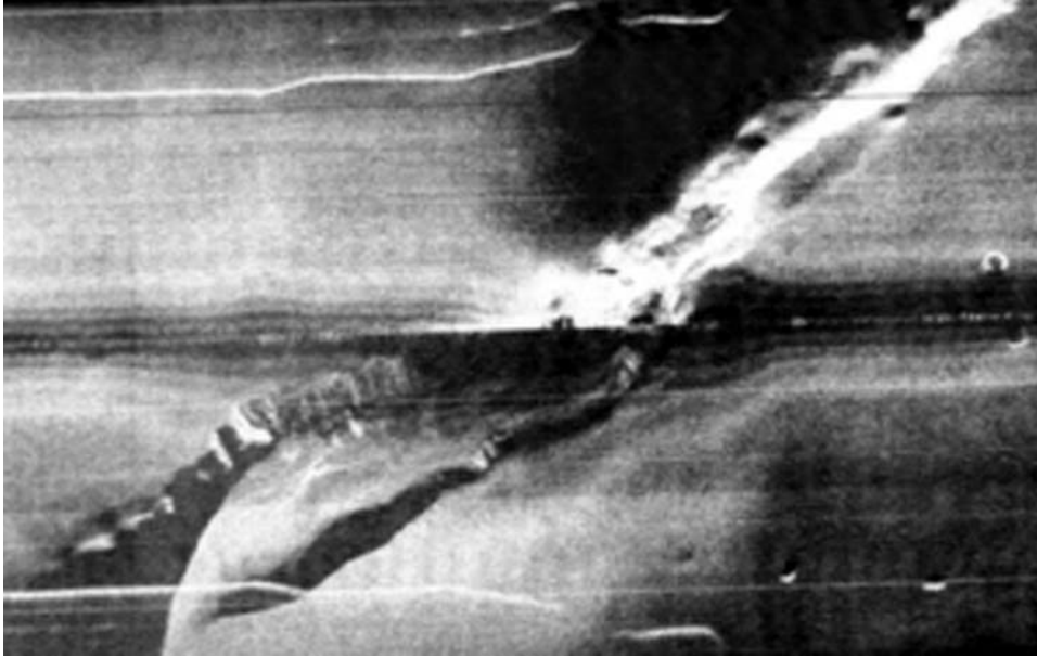
Figure 7.18. Uncorrected MAK-1 record of a fault scarp in the Mediterranean Sea. The image corresponds to a full MAK-1 swath and is 2 km wide (from Bejrdorff et al. , 1994; © UNESCO).
