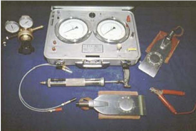
Figure 1.26 Dilatometer along with control panel and accessories (Courtesy of N.Sivakugan, James Cook University, Australia).
