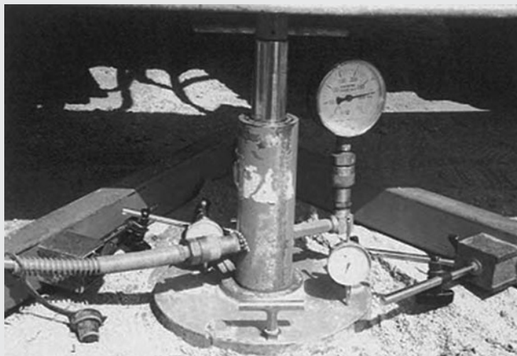
Figure 1.11 Plate load test in the field (Courtesy of Bjara M. Das, Henderson, NV).
