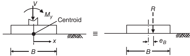
Figure 2.21 Eccentrically loaded spread footing.
