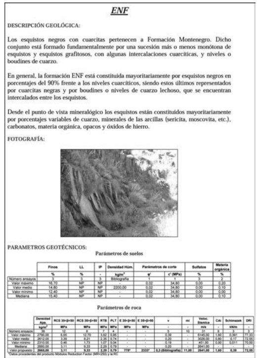
Figure 2. Example of 'fact-sheet' for the Black Schist formation in which the tunnels are excavated.
