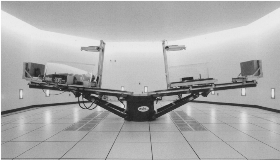
Figure 8.10. Research using NASA’s short-radius centrifuge may hold the key to realizing artificial gravity onboard future spacecraft. Image courtesy: Wyle.
