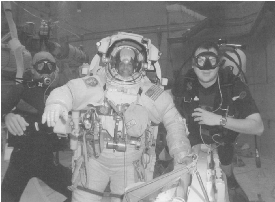
Figure 7.13. Divers assist astronauts during their simulated EVAs. Image courtesy: NASA ( see colour section ).
