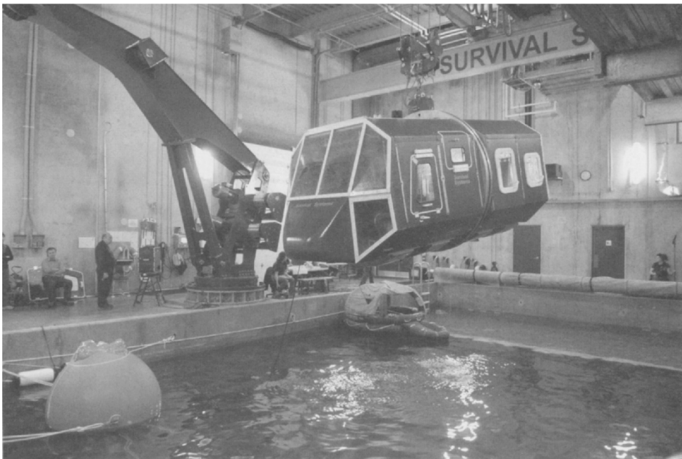
Figure 3.9. CSA astronaut applicants being evaluated inside Survival Systems' helo-dunker. Image courtesy: CSA ( see colour section ).
