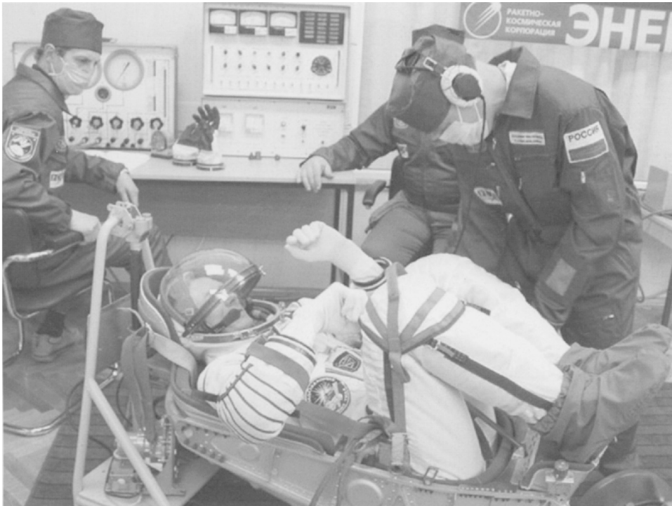
Figure 7.11. Engineers pour plaster into the Soyuz seat liner to ensure a comfortable fit. Image courtesy: NASA.
