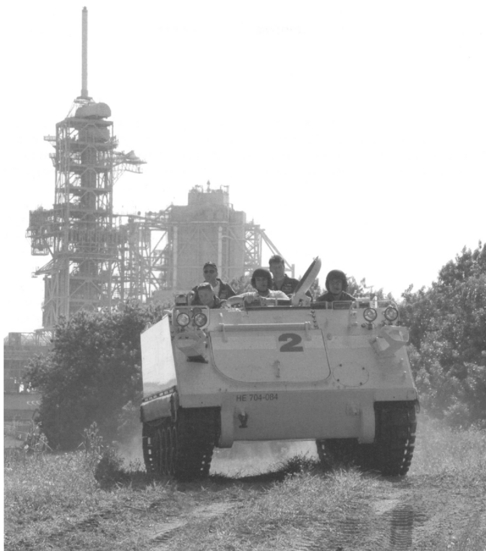
Figure 10.1. Astronauts put NASA’s M-113 escape tank through its paces before the Terminal Countdown Demonstration Test. Image courtesy: NASA.
