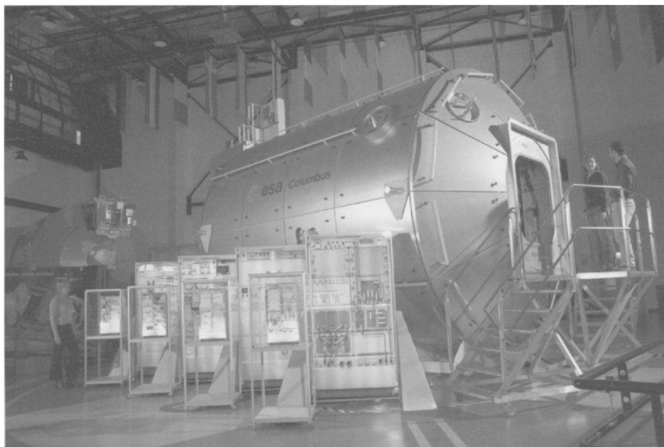
Figure 7.5. The Columbus laboratory mockup contains all the racks and experiment facilities currently mounted in the flight version docked with the ISS. Image courtesy: ESA (see colour section).
