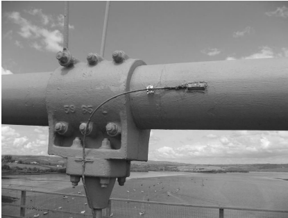
7.3 Fugro SMS sensors. (a) Cable tension; (b) wind speed and air temperature; (c) suspension cable temperature; (d) truss girder temperature.
