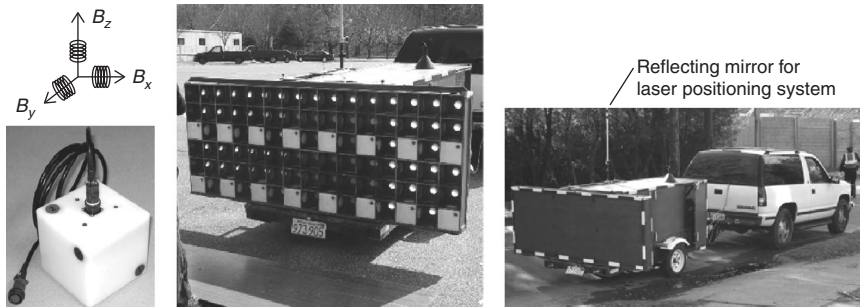
12.12 Magnetic field sensors in the dual-array system. (Left to right) Individual three-axis magnetometers; sensor layout; full system configuration for surveying.
