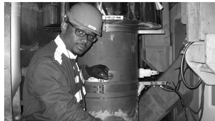
20.2 NDT techniques for NPP pipeline inspections: (a) Pipeline inspection using X-ray; and (b) P-scan inspection of a nuclear reactor.
