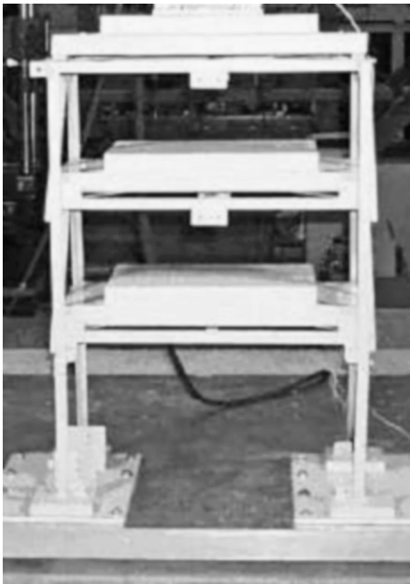
4.2 Three-story 1:10 scale building model.
