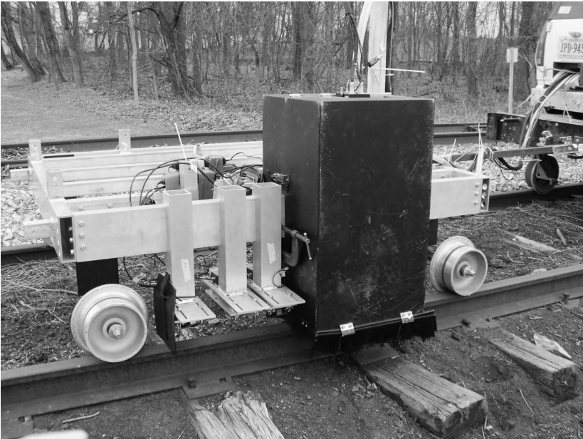
16.5 Early development of the UCSD laser/air-coupled system.
