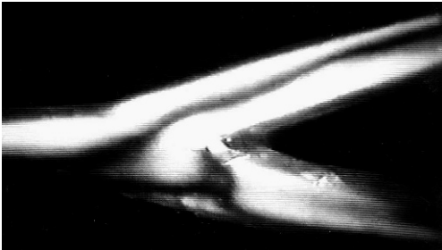
Fig. 12.58. Streamlines in an arterial branching with deposits and stress-optical visualization, Liepsch (1996)
