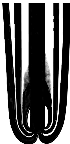
Fig. 7.16. Differential interferogram of the vertical heated plate, \text{Gr}_z = 8 \cdot 10^6
