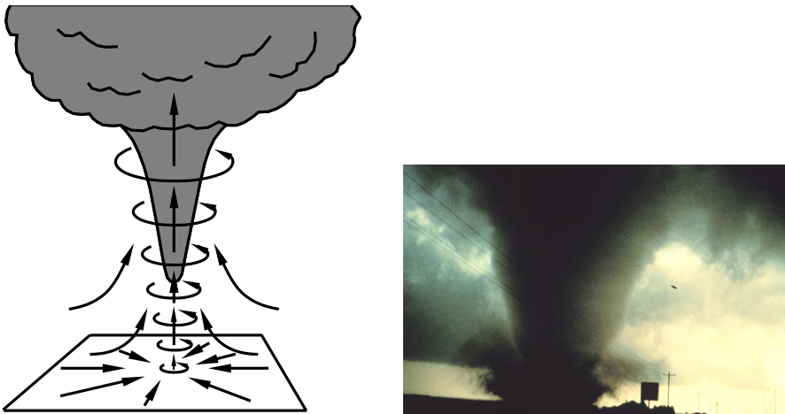
Fig. 10.17. Schematic representation of the vortex strength increase by means of horizontal flow convergence. The funnel-like protrusion of the cloud (shaded) corresponds approximately to the visible part of a tornado (right picture)
