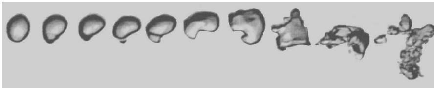
Fig. 8.8. Sequence of different bubble forms until bubble decay, under the effect of a turbulent liquid flow, F. Risso and J. Fabre (1998)
