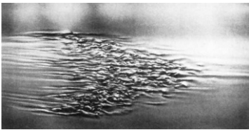
Fig. 6.26. Turbulent spot, R. Falco (1980)
