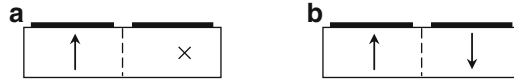
Fig. 10.10 Transducer designs: (a) NPSAVP-1, (b) NPSAVP-2; polarization directions are shown by arrows, depolarization zone is marked by the cross
