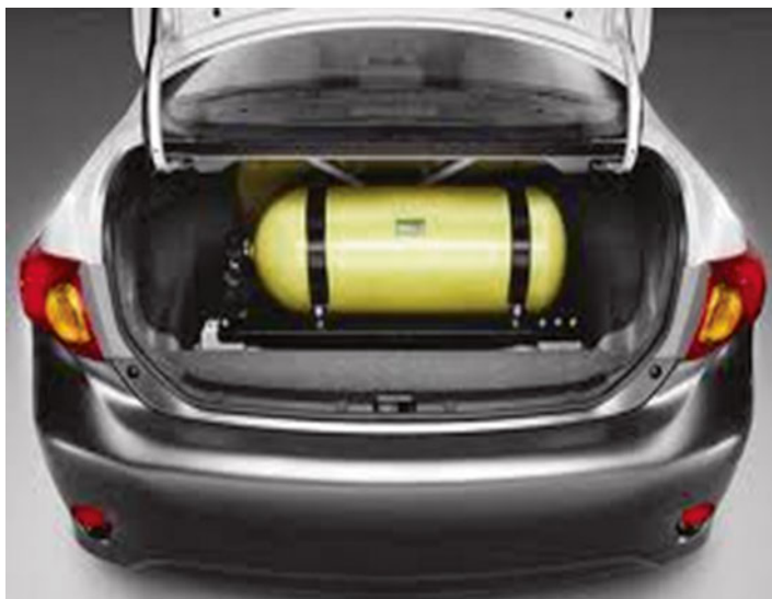
Fig. 3 Car with CNG conversion kit (Source: http://naturalgasconversion.net/ )
