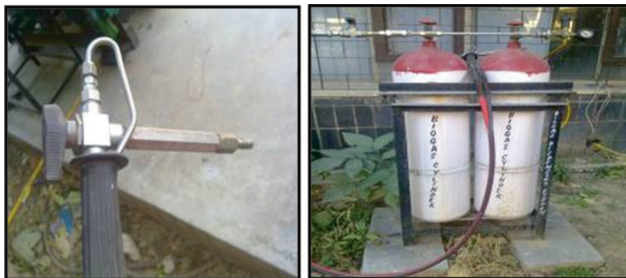
Fig. 7 Upgraded compressed biogas dispensing nozzle and a two-cylinder CNG cascade
