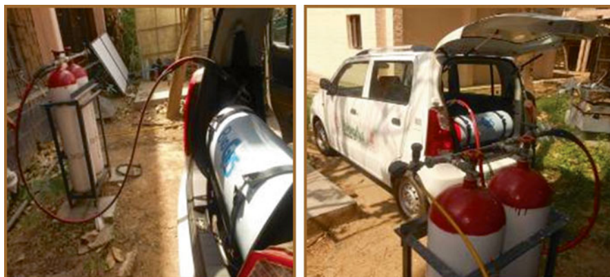
Fig. 9 Upgraded biogas dispensing system being used to fill biogas vehicle demonstrated at IIT Delhi
