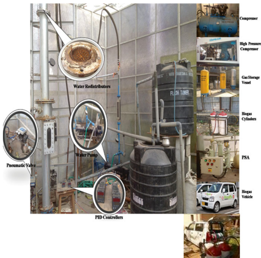
Fig. 5 Modified purification plant
