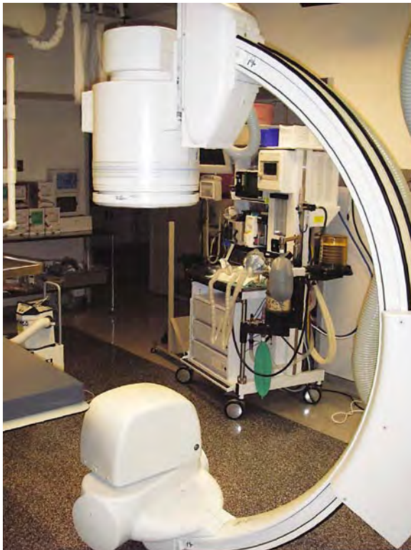
Fig. 7.51. C-arm mounted image intensifier of its last generation. This system has been used for rotational angiography and 3D-DSA since its introduction in the late 1990s (see examples in Figs. 7.70–7.73, 7.81, 7.83, 7.85)
