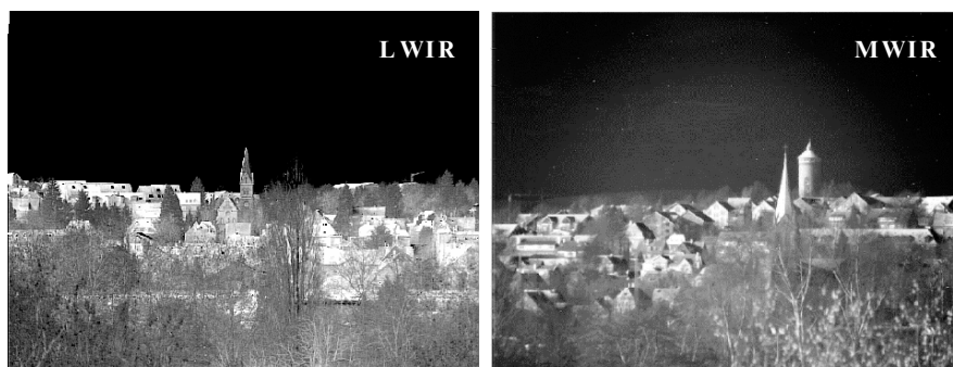
Fig. 9.6. 640 \times 486 thermal images taken by a low-noise QWIP camera ( left ) and by a MWIR QWIP camera ( right ) [18]
