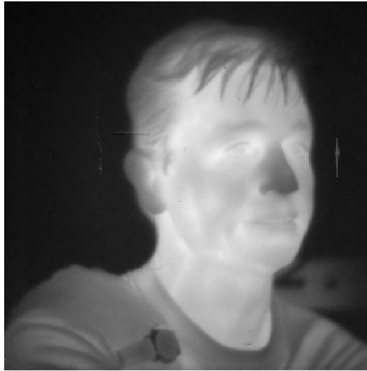
Fig. 8.22. Thermal image of a person (See Dupont et al. [191] for details)
