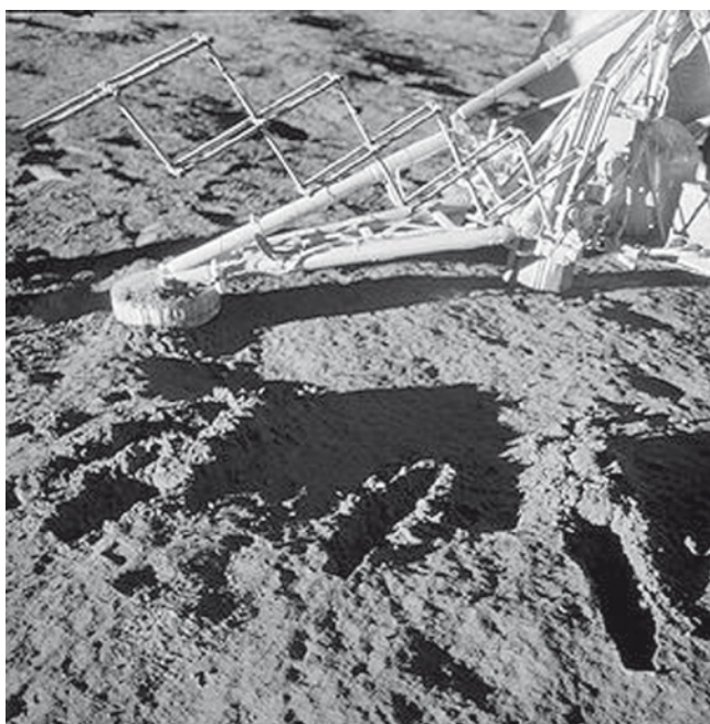
Fig. 23.3 Surveyor 3 deploying shovel (NASA).
