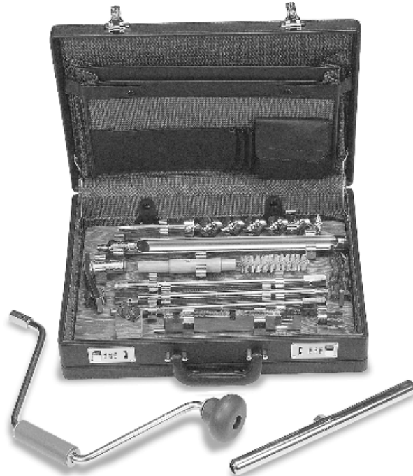
Figure 3-15. Split-spoon sampler with extension rods for deep samples. (Courtesy of Forestry Suppliers, Inc., http://www.forestry-suppliers.com .)
