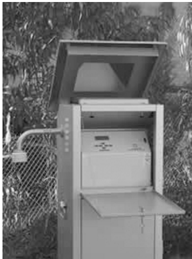
Figure 3-3. HV3000 high-volume air sampler designed by Ecotech Pty Ltd, Blackburn, Victoria. (Reproduced with permission from Ecotech Pty Ltd, http://www.ecotech.com.au/hv3000.htm .)
