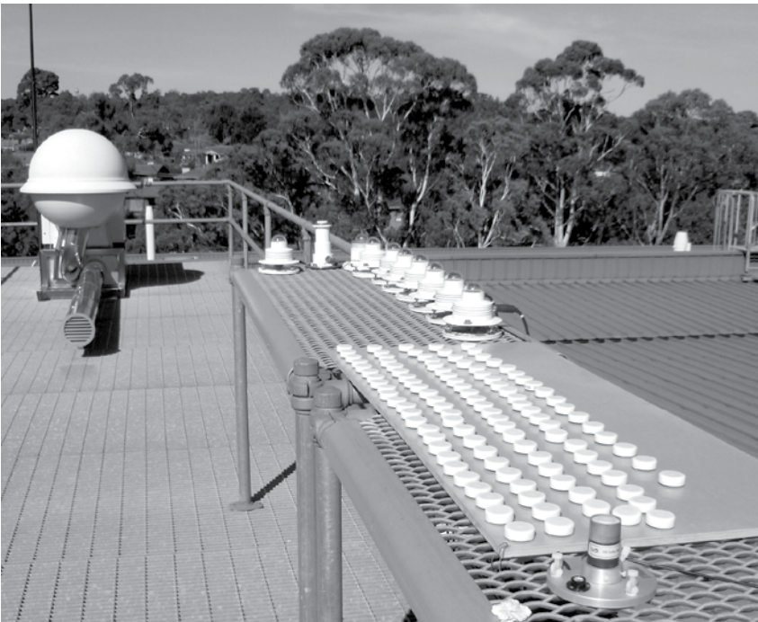
Figure 7.6 A large batch of personal UV Dosimeters on the roof of the ARPANSA Laboratory undergoing calibration against the calibrated ARPANSA traceable Bentham spectral system.
