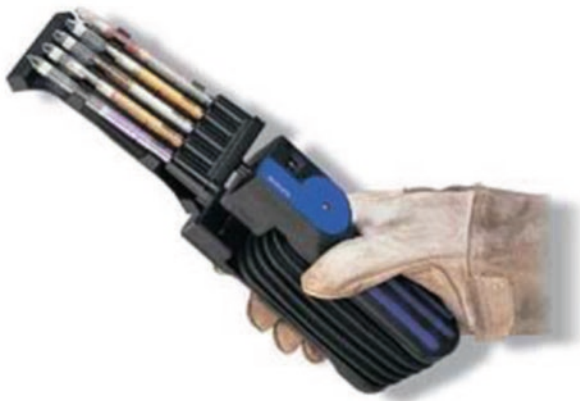
Fig. 3.20 The simultaneous test sets manufactured by Dräger safety (Lübeck, Germany) (Adapted from Ref. [53])
