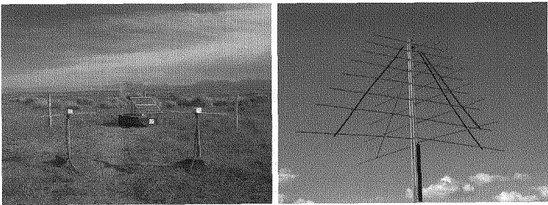
Fig. 1. Left: A standalone antenna setup near the center of the Pierre Auger Observatory. Right: LPDA antenna used to obtain the results presented here.
