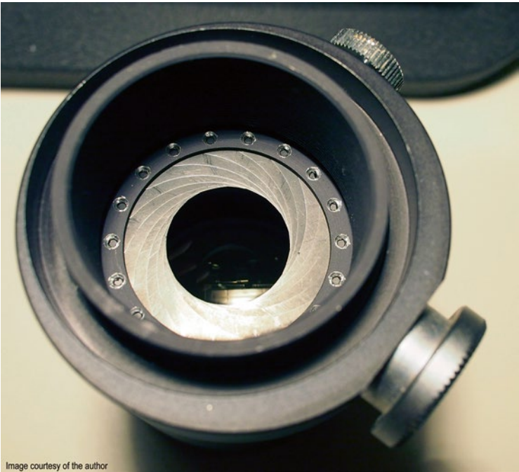
Fig. 1.20 High quality construction showing 18 blade diaphragm
