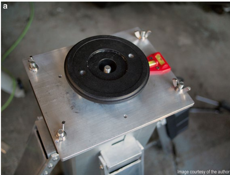
Fig. 5.16 Homemade top plate for mounting of EQ6
