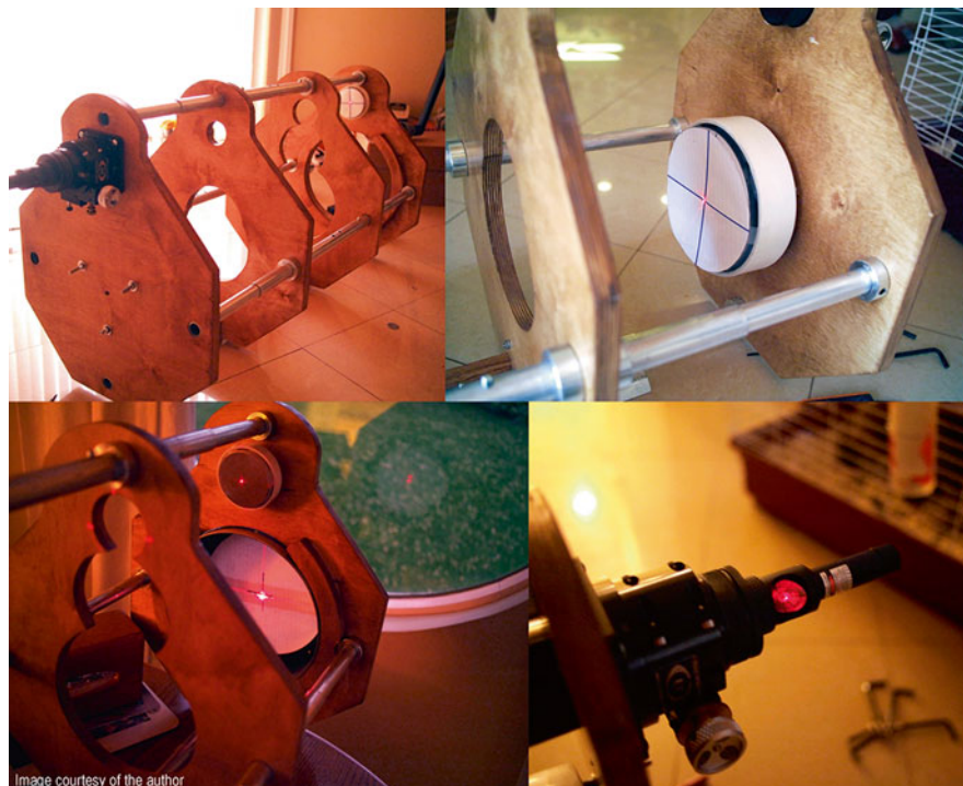
Fig. 4.4 Collimation of folded refractor using paper circles with marked centers
