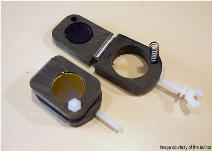
Fig. 4.66 Housing showing flip movement in pitch axis with spring loaded nylon threaded machine screw
