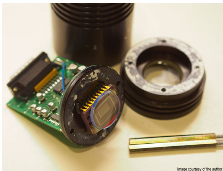
Fig. 3.10 Dissected Starlight Express HX916 camera wearing Newport Optics flattening lens
