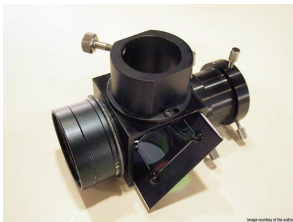
Fig. 2.20 ONAG being assembled
