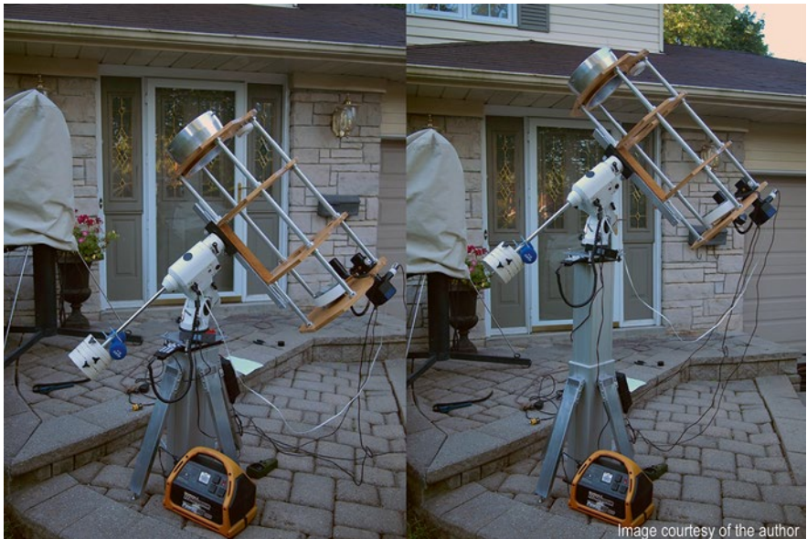
Fig. 5.17 Electrically powered variable height pier in action
