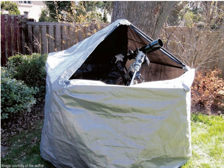
Fig. 5.24 Finished dome with zippered opening revealed and one strut removed to allow telescope viewing or imaging
