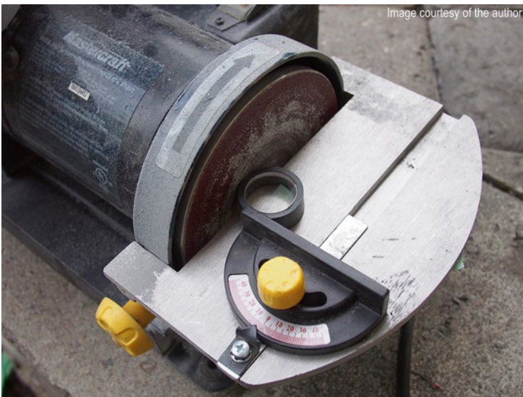
Fig. 5.3 Shaping prism retaining rings to fit Meade Barlow
