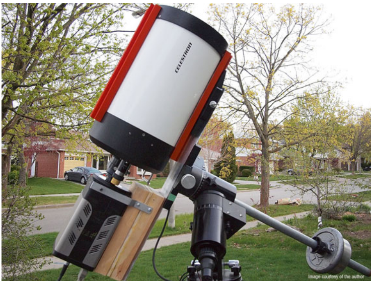
Fig. 2.28 PhotoMax EMCCD mounted in tandem with 8" Celestron SCT. Why is this Celestron SCT white? Back in the 1990s Vixen and Celestron shared product line but often sold each other's items in their own colors. Black Vixen manufactured fluorite refractors bearing the Celestron name are common second hand finds. Apparently Vixen sold white 8" SCTs in Japan. This SCT was a special order, painted white at the factory but sporting Celestron labels
