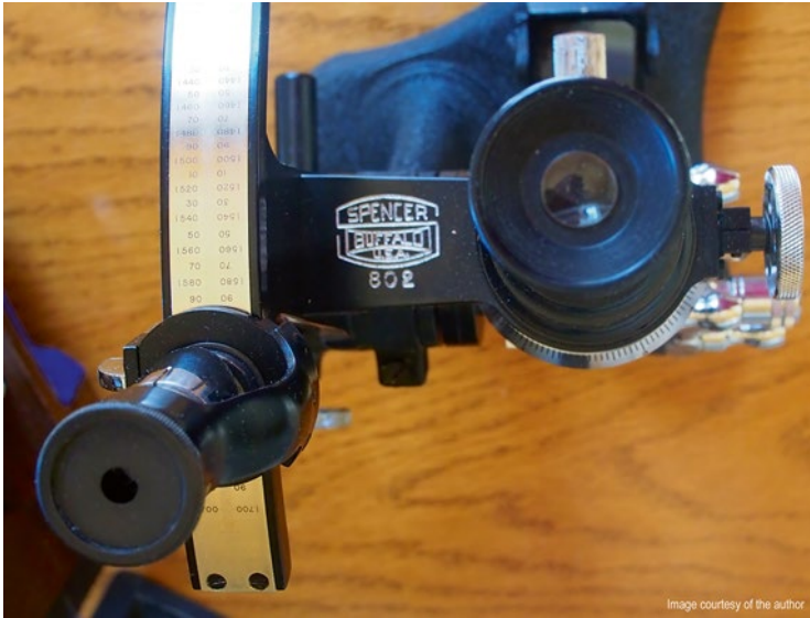
Fig. 1.37 Reading the index of refraction scale on refractometer
