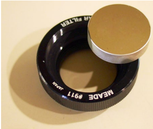
Fig. 5.28 Return beam optical flat installed in empty SCT filter ring
