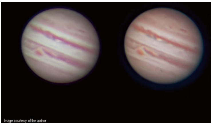
Fig. 4.12 Jupiter imaged with PGR Flea3 at f/30 ( left ) and with Chromacor-N ( right ). Significant correction to color fidelity and increased detail shown on right image . Even though CA is not readily apparent visually these images show how much detail and resolution is lost with an achromatic refractor, you just don't realize it
