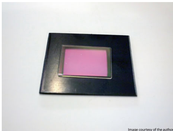
Fig. 2.19 Carl Zeiss FT660 DRLP epoxied onto flip mirror stop
