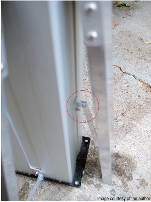
Fig. 5.15 Retracted leg with collapsed strut
