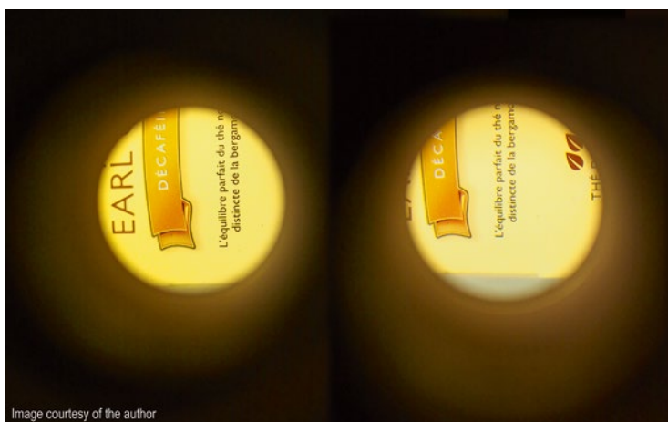
Fig. 5.6 Image shift as correction is enabled on ADC
