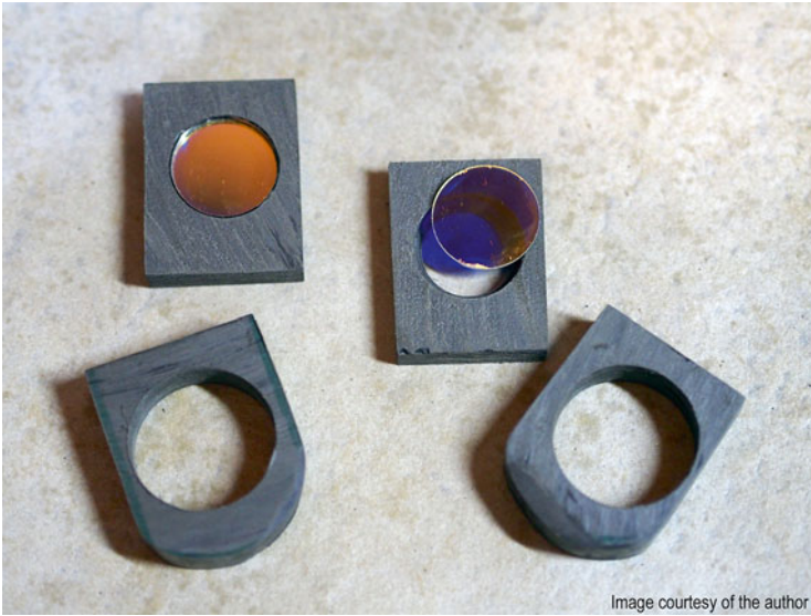
Fig. 4.65 Omega Optics solid Fabry-Pérot etalons and custom polycarbonate housings
