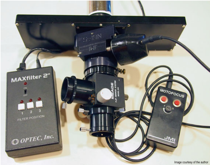
Fig. 2.2 Jim's Imaging Train: Optec powered 2" RGB filter slide, JMI NGF-S motorized crayford focuser, Meade 644 flip mirror. On Newtonians, typically there is insufficient focus travel to incorporate the flip mirror so a good illuminated finder with a multiple etched reticle can be used to accurately position the planet. Surplus Shed and eBay are good sources for these reticles
