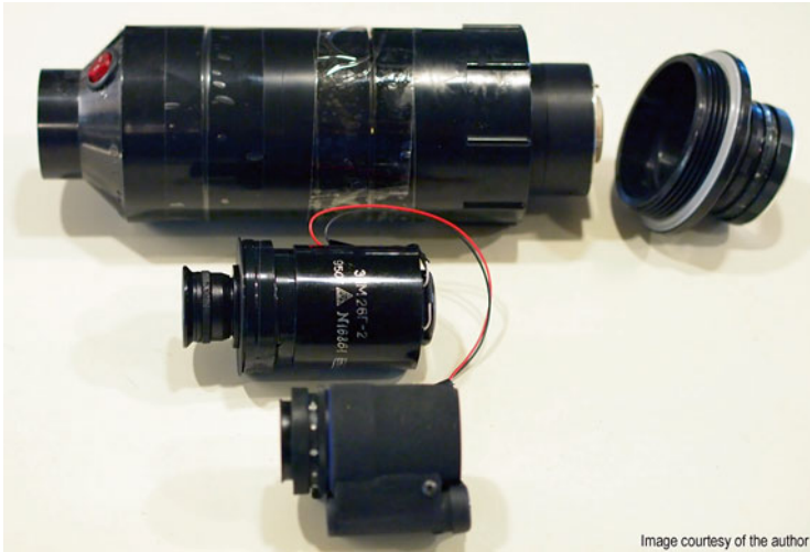
Fig. 3.24 Three generations of image intensifiers from top to bottom : E2V P8079HP, ROMZ Rostov Cyclop 11B2, Generation 3 thin film monocular
