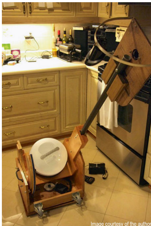
Fig. 4.31 Cake lid covering mirror. Secondary mirror diagonal suspended on a single curved spider made from hand bent aluminum bar
