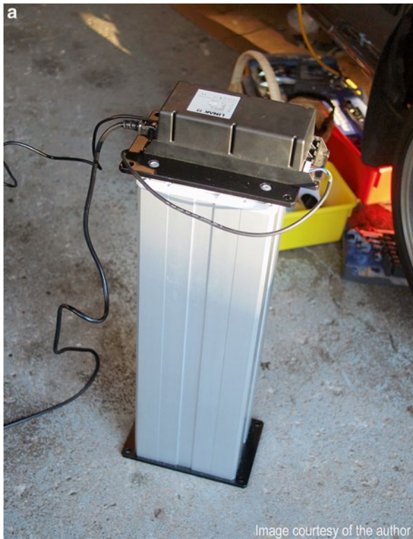
Fig. 5.8 Linak Desklift DL2 with control box on top in retracted and fully extended positions
