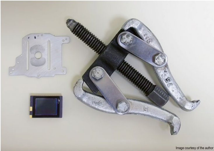
Fig. 1.33 Gear puller used to remove bonded KAF8300 sensor from aluminum board
