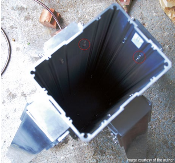
Fig. 5.13 Leg hinge mounts fixed to outer extrusion via flat head machine screws placed in recessed surfaces of the extrusion. Inner extrusion is able to pass without interference
