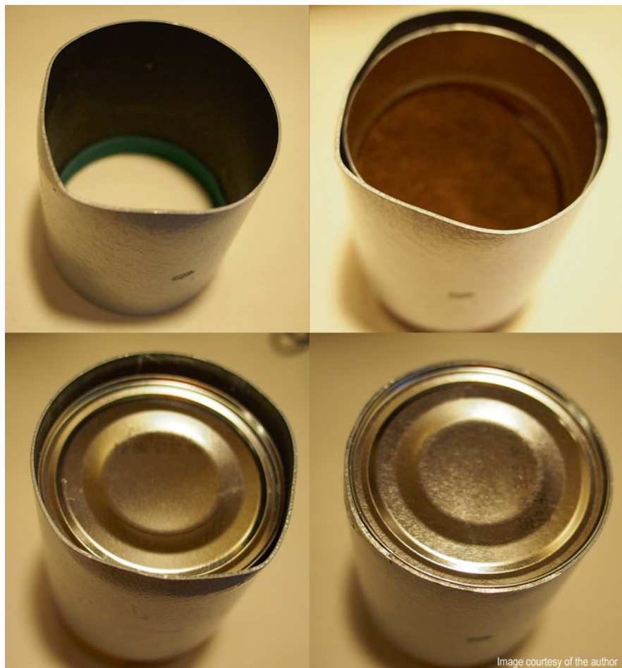
Fig. 4.50 Dented dew cap being restored with perfect fit can of ground coffee
