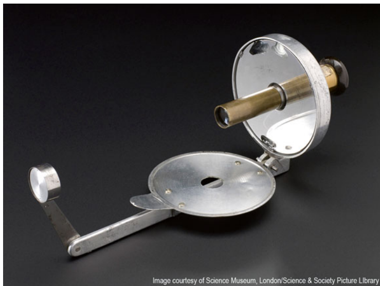
Fig. 4.34 Horace Dall's folding cassegrain reflector, the ultimate expression of elegant minimalism
