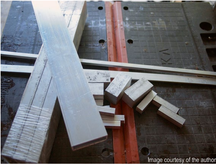
Fig. 5.10 Aluminum from metalsupermarket.com, 1"×1"×2" blocks for the leg hinges, 1"×2"×20" hollow pieces for the legs
