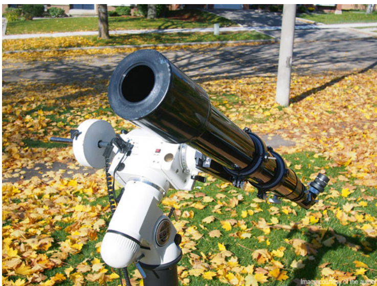
Fig. 4.69 Celestron 90 mm, f/11 achromat stopped down
