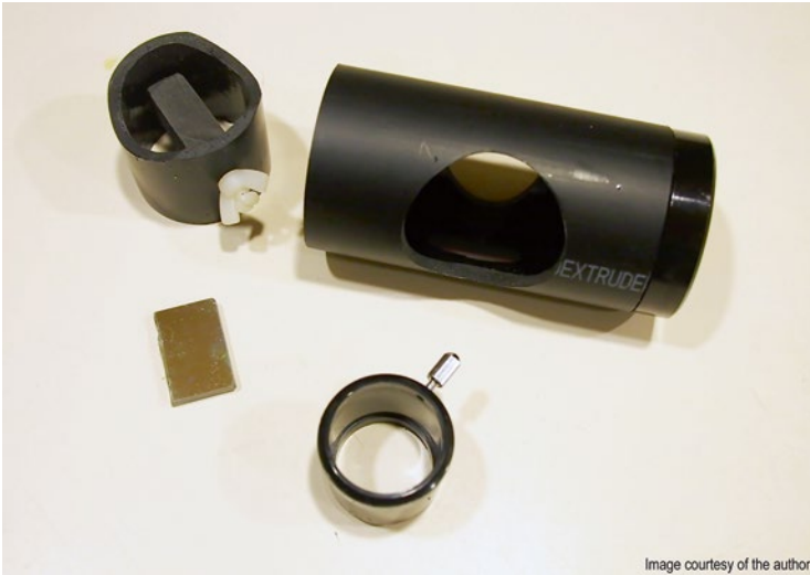
Fig. 5.33 Black PVC pipe fiber optic housing and off axis eyepiece/guide camera viewer
