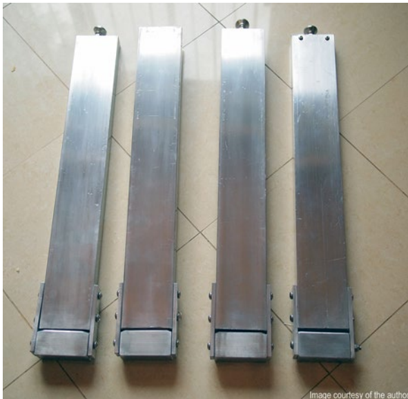
Fig. 5.11 Solid aluminum bar was driven by force into the ends of the legs and threaded leveling feet attached
