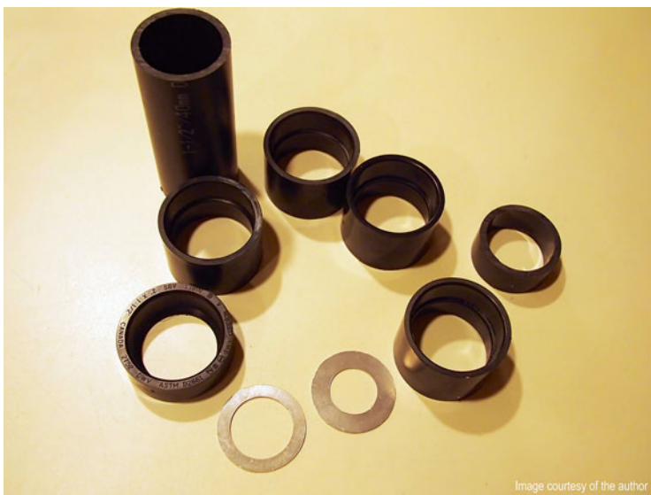
Fig. 4.36 Baffle tube components from plastic plumbing pipes
