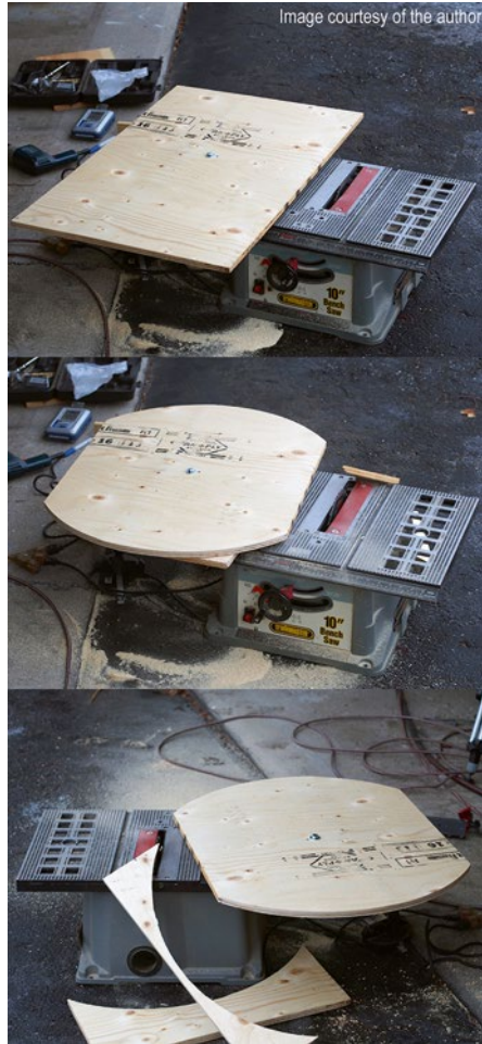
Fig. 5.53 How to cut large perfect plywood circles on a miniature table saw
