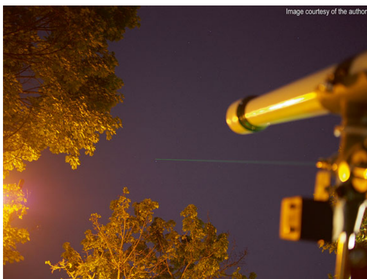
Fig. 4.57 Hotech green laser aligning ATCO mount with Polaris
