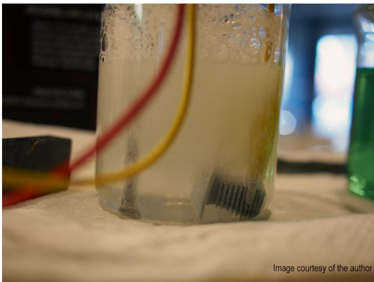
Fig. 4.59 Electrolytic rust removal of CGE bolt
