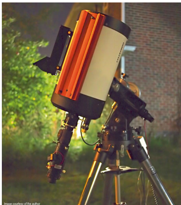
Fig. 3.33 Celestron 8" SCT operating at f/1.7 with coupled Gen3/Gen2 image intensifier
