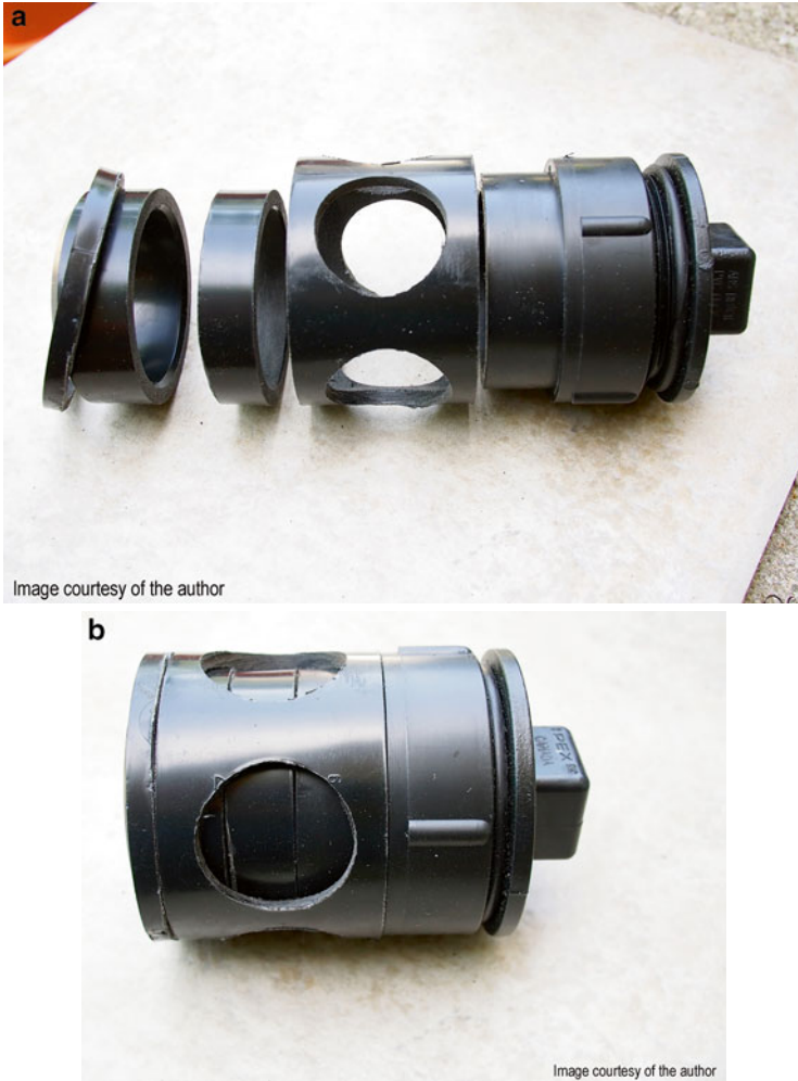
Fig. 3.17 A final end ring is from the same material used to make the rotating sleeve and when the pieces are glued together will prevent the sleeve from coming off
