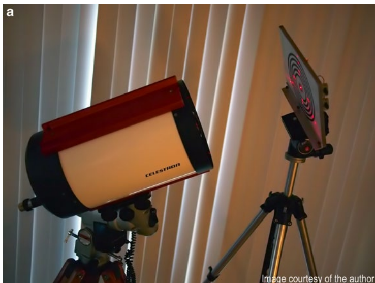
Fig. 5.27 Orthogonal centering of Jim's CT Laser Collimator with C8 primary mirror
