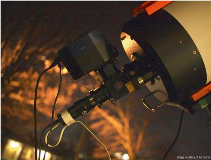
Fig. 2.21 Imaging the Eskimo Nebula at f/10 on 8" Celestron SCT. Bonus points to those who can explain why the Celestron SCT is white (this is the OEM factory paint) and not black, grey or orange. The SCT dates back to the 1990s
