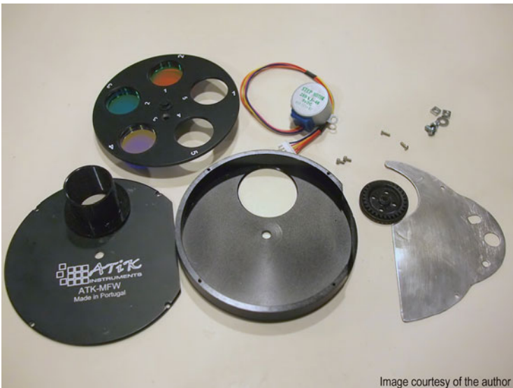
Fig. 2.3 Build your own motorized filter wheel, a project in progress. A manual 5 position 1.25" filter wheel with 28BYJ-48 stepper motor and ULN2003 driver and Arduino, no motor shield needed
