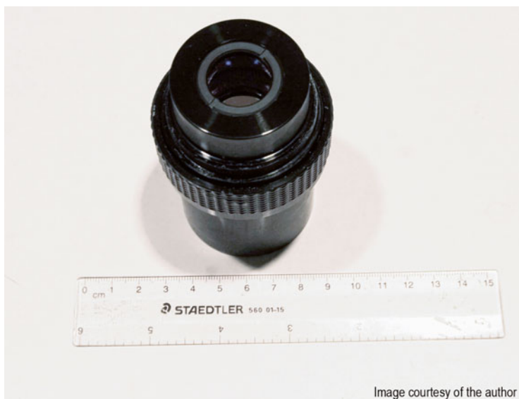
Fig. 3.2 The 20 mm aperture PST air space etalon with 2" adaptor attached
