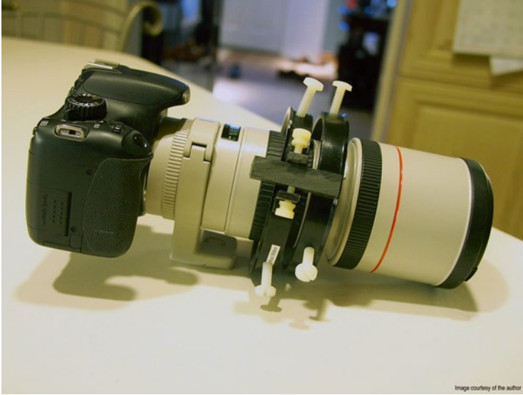
Fig. 1.23 Fine lens focuser mounted on Canon EOS 300 mm f/4 L lens
