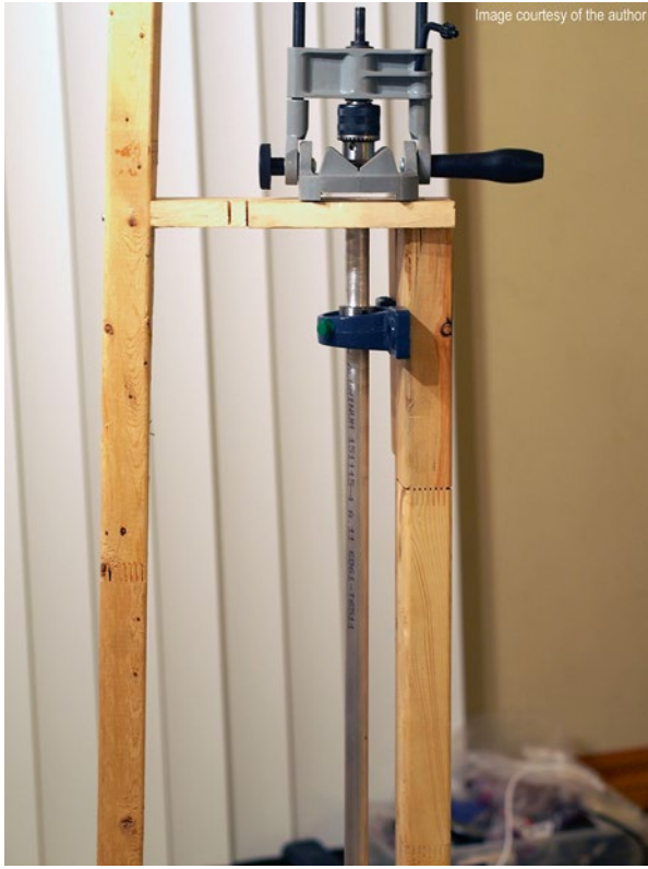
Fig. 5.58 Tapping threads into one of the aluminum bars
