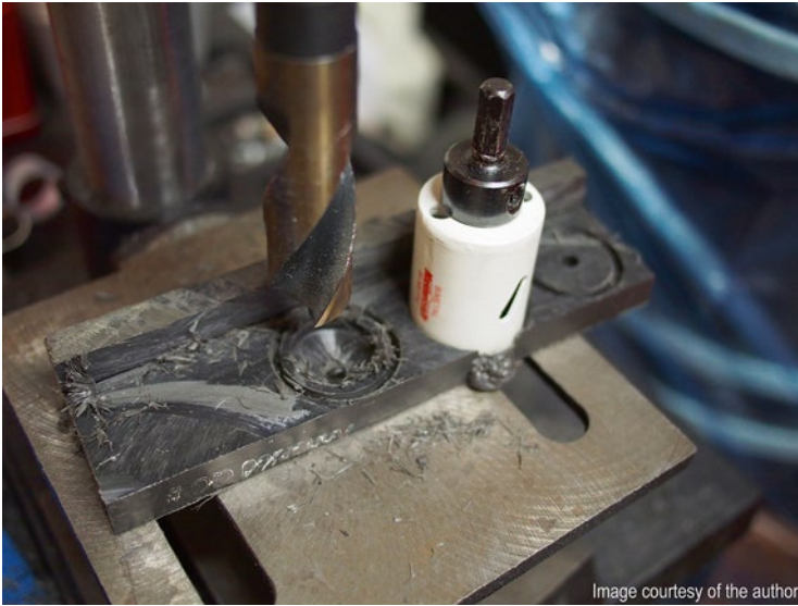
Fig. 5.2 Cutting prism retaining rings from polycarbonate
