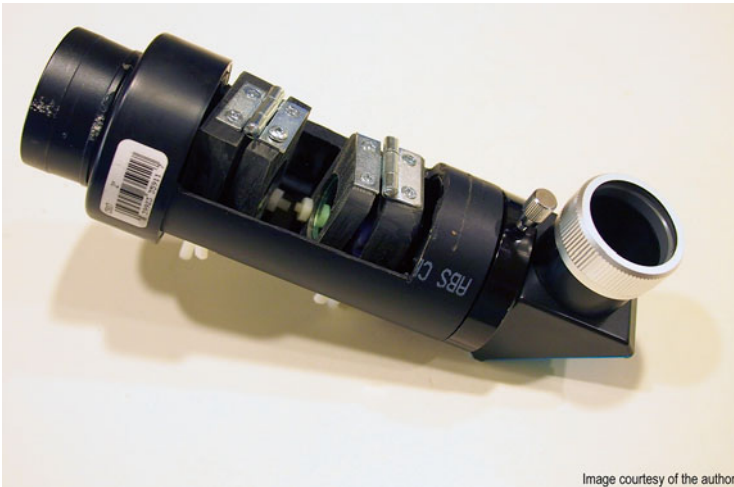
Fig. 4.67 Completed module with 1.25" diagonal and 2" nose. Open access allows rotation and tilt adjustment of filters
