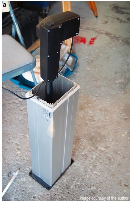
Fig. 5.9 Linear actuator controls DL2 movement with its actuator extension bolted to the bottom plate. When it extends, its body pushes against the top plate and the inner aluminum extrusion rises. The inner and outer extrusions are engineered to tight tolerances, the inner extrusions has fixed runners traveling up and down the corrugated channels of the outer extrusion to guide its movement and maintain stability
