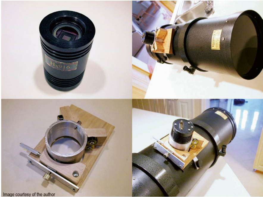
Fig. 3.11 Three inch monster crayford focuser construction
