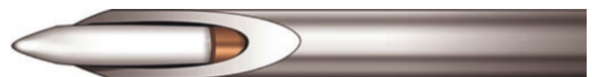
Fig. 12.2 Close-up of the distal portion of the injector. The implant is contained in the needle in the distal portion of the injector
