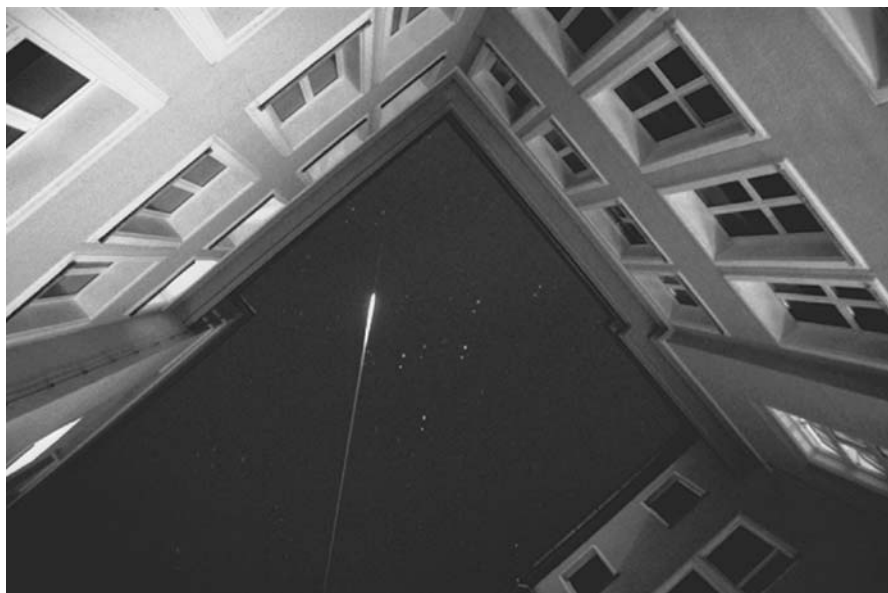
Fig. 14.1. White-light filament generated in the atmosphere by infrared femtosecond-terawatt laser pulses. (Photo C. Wedekind)
