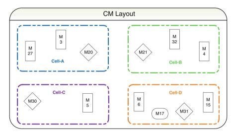
Fig. 17.2 Machine allocation in cellular layout
