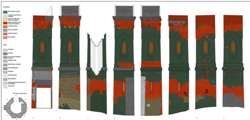
Fig. 19.3 East tower, exterior fronts: mapping of materials and decay phenomena
