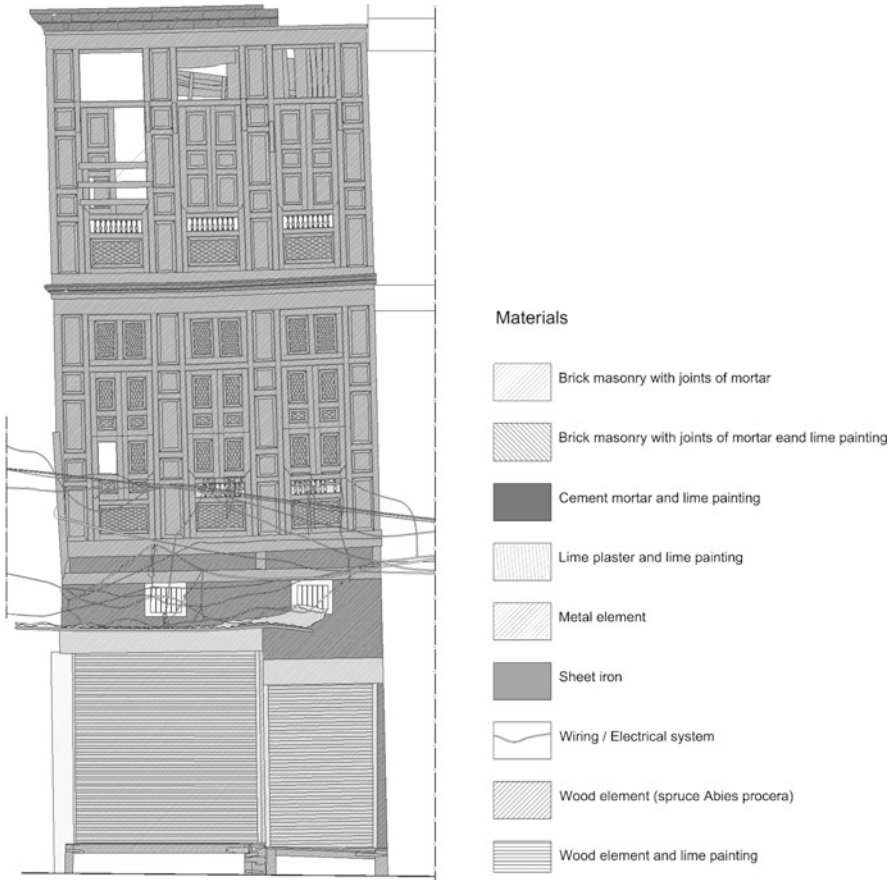
Fig. 18.7 Material survey—facade on the Haram Street Bazaar
