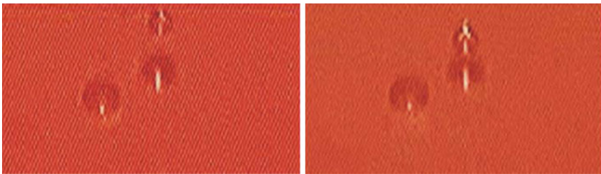
Fig. 4.18 Observation of axial bistability in the optical binding of two aqueous aerosol droplets in optical tweezers
