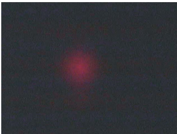
Fig. 5.17 A fluorescence image of a decane droplet loaded with quantum dots
