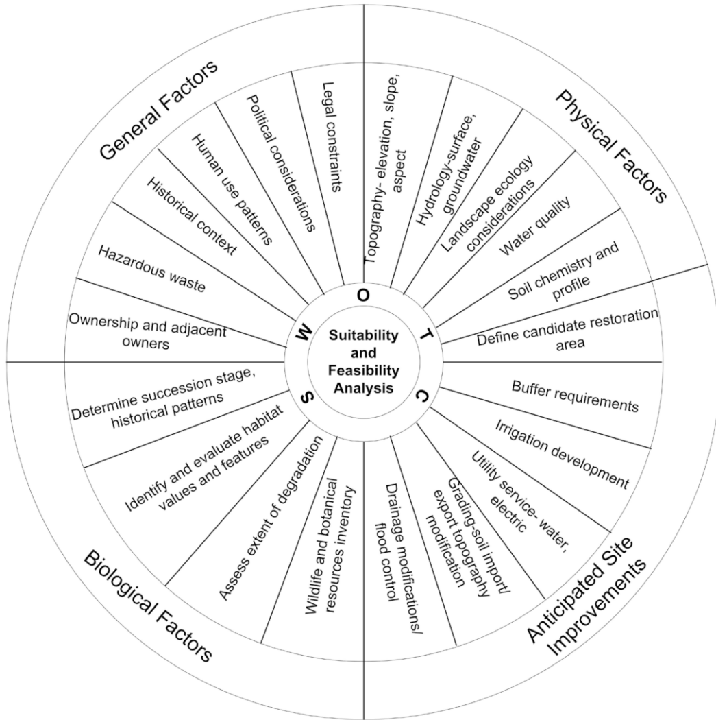
FIGURE 4-1. Site analysis factors by category used in the feasibility analysis process.
