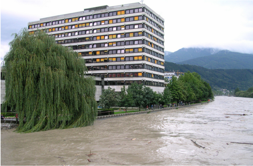
Fig. 2.2 The flood in Innsbruck on August 23, 2005. The discharge at the time (4.48 p.m.) the picture was taken was at around 1,395\text{m}^3/\text{s} . Only a few centimetres of freeboard are protecting the city of Innsbruck and the university (picture) from catastrophic damage
