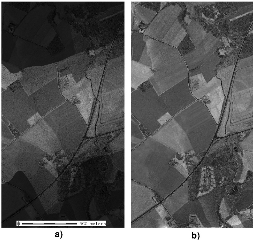
Fig. 11.5 Digital Intensity Models: a) uncorrected DIM representing original recorded intensity values and b) DIM corrected for influences of scan geometry, topography and atmosphere
