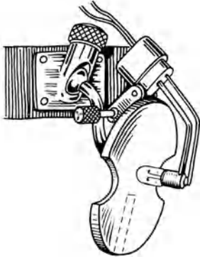
Fig. 24. Headlight by BRÜNINGS-PERWITZSCHKY with lateral notches in mirror for use as with CLAR lamp. Dotted line on mirror: slit for direct.
