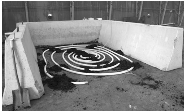
Fig. 22.6. Spiral aeration system of a fungal pilot pile. It can be connected to a compressor for continuous active aeration
