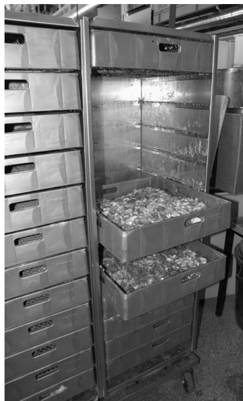
Fig. 22.1. Bark material, which was pre-steamed, inoculated and pre-grown in a stainless steel chamber of 2 m 3 volume. It served as inoculum for fungal tubes
