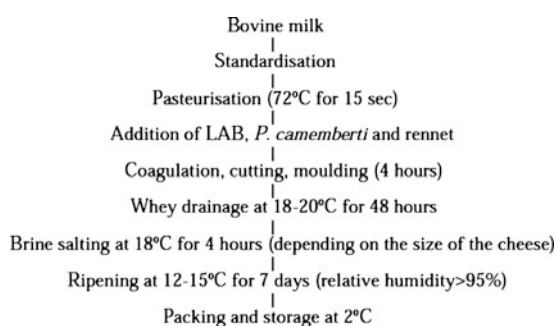
Fig. 1.5. Flow diagram for the production of Camembert/Brie
