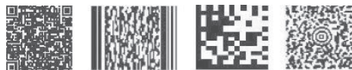
Figure 2. 2D Codes in ISO/IEC Standards: (From left) (a) QR Code (ISO/IEC 18004); (b) PDF417 (ISO/IEC 15438); (c) Data Matrix (ISO/IEC 16022); (d) Maxicode (ISO/IEC 16023)
