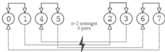
Figure 7: Illustrates the first n/2-1 exchanges of the N-Body algorithm with an optimal configuration. When n=8 , there are three such passes, each with two overlaps resulting in a total of 6 messages crossing the hot spot.
