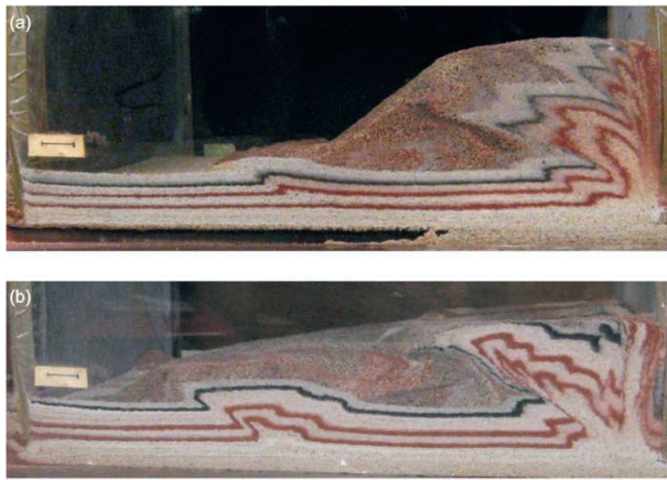
Fig. 3.37 Effects of surface erosion on localisation of exhumation in experimental thrust wedges. (a) High and (b) low basal friction ( referred on page 60 )
