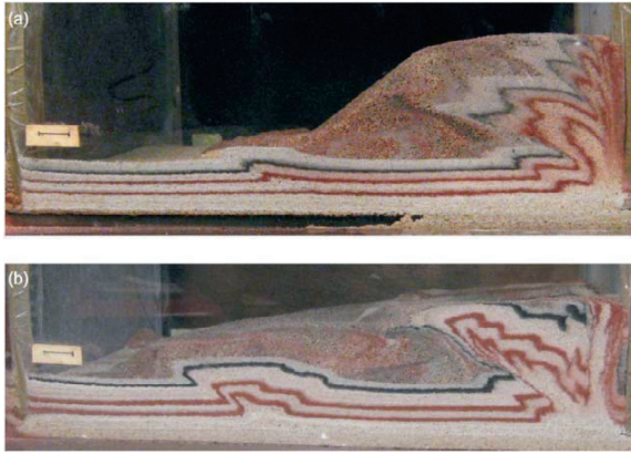
Fig. 3.37 Effects of surface erosion on localisation of exhumation in experimental thrust wedges. (a) High and (b) low basal friction
