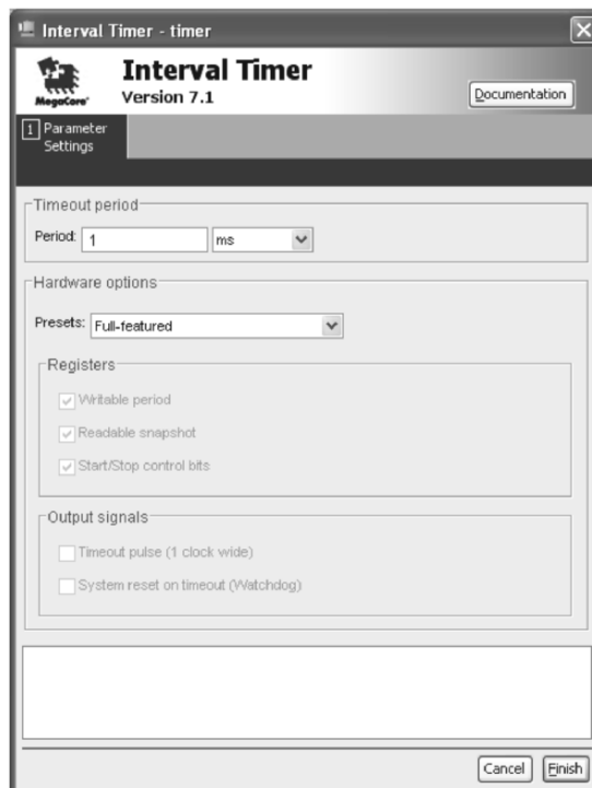
Figure 17.8 These are the settings for the interval timer device to be added to the Nios II system.
