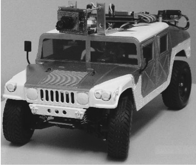
Figure 13.25 Hobbyist R/C model with a CMU camera and R/C PWM servos controlled by an FPGA
