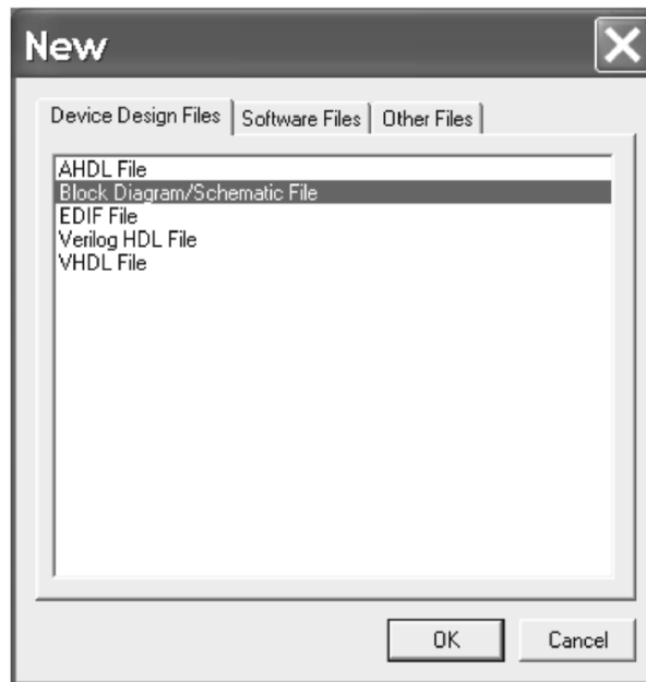
Figure 1.10 Creating the top-level project schematic design file.
