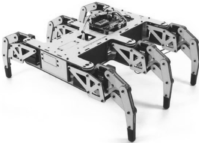
Figure 13.26 Lynxmotion Hexpod Walking Robot Kit with 12 R/C servos
