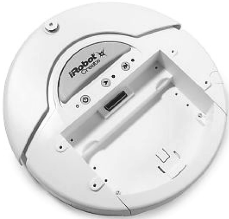
Figure 13.28 iRobot's iCreate robot base can be controlled by an FPGA with a Nios Processor using an RS-232 serial port to send commands to the iCreate robot's internal microcontroller. Photograph courtesy of iRobot.
