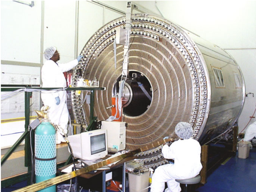
Fig. 7.20 The Central Outer Tracker of the CDF experiment. Reprinted from [13] with permission
