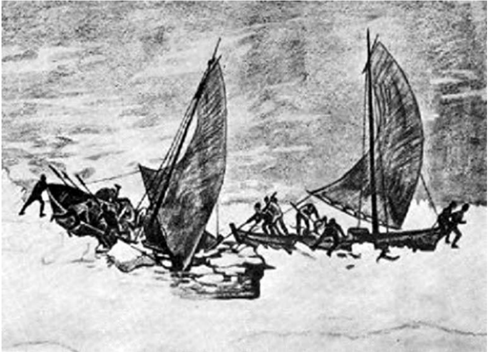
Figure 1.2. Postal route across the Åland Sea in 1638–1895. Peasants in Eckerö, Åland designed a mail boat for the difficult drift ice conditions, to cross leads, new ice, thick ice, and ridged ice. This system ceased when steamboats were introduced to provide the service. (Watercolor painting by J.A.G. Acke, 1909, reproduced by permission of the Åland Museum of Art, Finland.)
