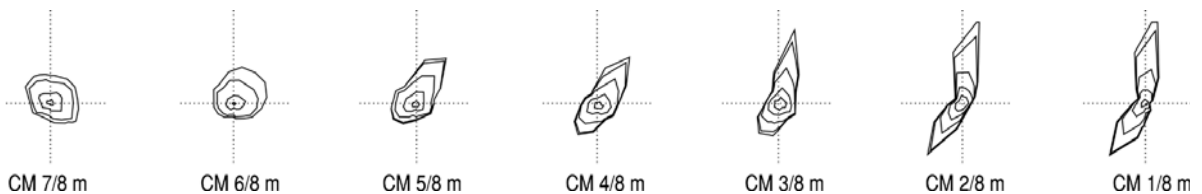
Figure 5.8. Current roses based on measurements outside Rauma, Sea of Bothnia during the International Gulf of Bothnia Year 1991. The graphs describe the cumulative probability of current speeds at 5 cm/s spacing in different directions. Station CM1 is closest to the coast (10 km) whereas Station CM7 is 55 km from the coast. The x -axis is directed to the east and the y -axis to the north. The measurement depth is 8 meters. (Murthy et al. , 1993.)
