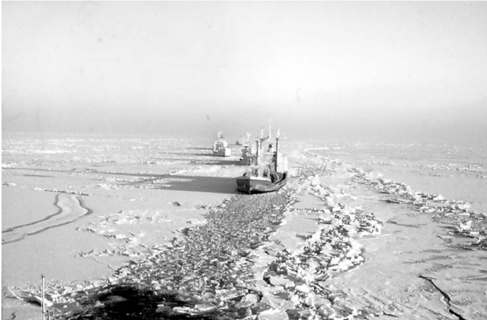
Figure 7.20. Convoy of ships assisted by an icebreaker in the Baltic Sea. Ice dynamics determines the length of the convoy that can follow an icebreaker.
