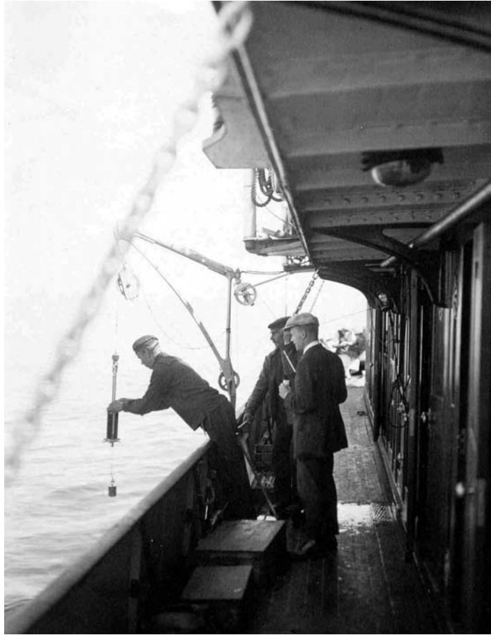
Figure 3.13b. Hydrographic surveying aboard R/V Nautilus using Nansen bottles. (Courtesy of the Finnish Institute of Marine Research.)
