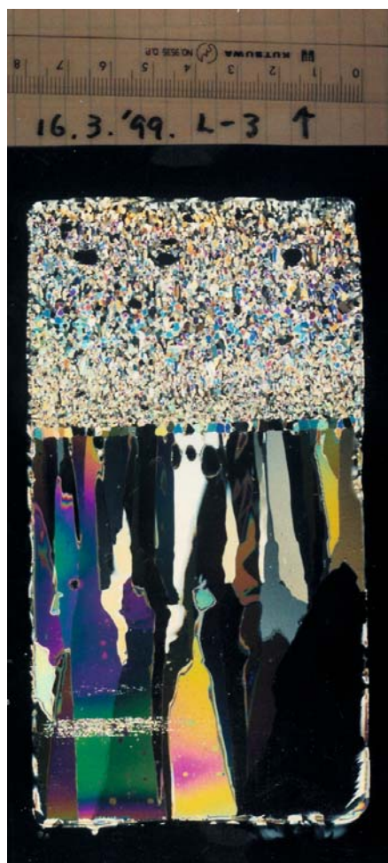
Figure 7.4. Ice crystal structure in Baltic Sea ice (left) and lake ice (right). The top layer is fine-grained snow ice, and the lower layer is columnar-grained congelation ice. (Prepared by Dr. Toshiyuki Kawamura, printed by permission.)
