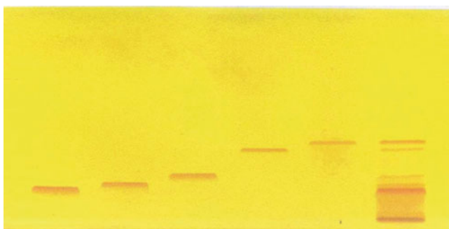
Fig. 14.18 HPTLC chromatogram by AMD of opium extract and standard alkaloids of opium: (1) morphine; (2) codeine; (3) thebaine; (4) papaverine; (5) noscapine; (6) opium extract; eluent used was universal gradient: methanol 100, methanol-dichloromethane 50/50, dichloromethane 100, dichloromethane 100, hexane; 100; derivatization by Dragendorff reagent. [From Pothier and Galand (2005) with permission]
