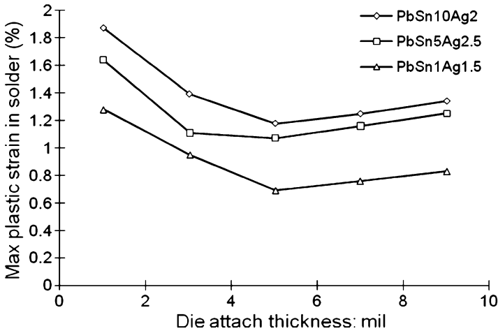
Fig. 5.35 The maximum effective plastic strain in die attach solder vs. die attach thickness
