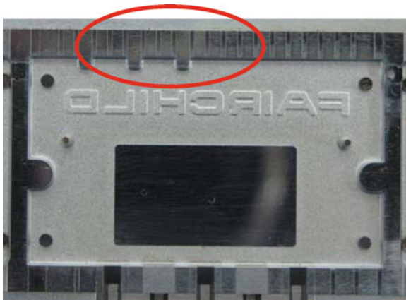
Fig. 8.58 A picture of the cavity of in a mold die (© 2008 IEEE)
