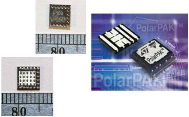
Fig. 3.15 Multiple direction heat transfer packages
