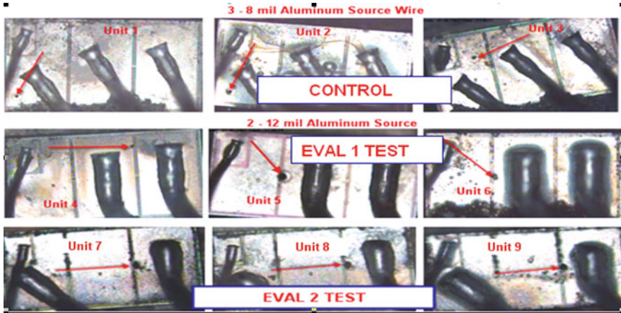
Fig. 12.48 FA decap (actual photo) for UIL failures after characterization
