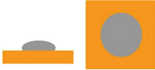
Fig. 9.50 Melt solder on DAP of a lead frame
