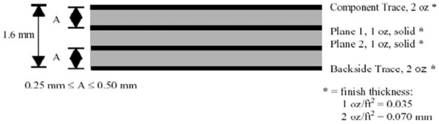
Fig. 6.14 Cross section of multilayer PCB in JEDEC standard 6.15 SOP test board (pitch: 1.27 mm)
