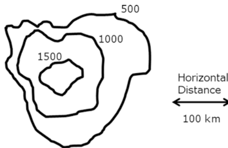
Fig. 3.1 Contours of elevation (m) above sea level of a mountain. The contour interval chosen is 500 m. Where are the steepest parts of the mountain? Can you climb the mountain by following a contour line?
