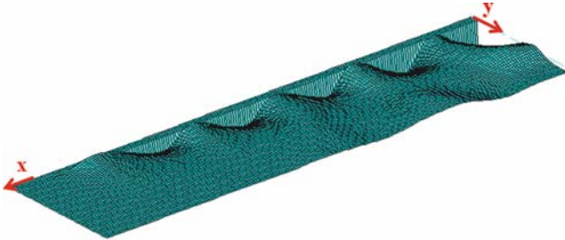
Fig. 6.1 Exercise 15. Snapshot of the deformation of the sea surface caused by a coastal Kelvin wave in the northern hemisphere
