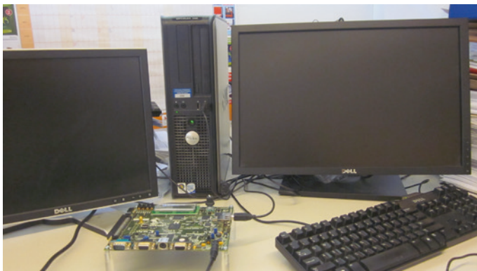
Fig. 5.44 Photograph of FPGA board with PC connection through USB cable
