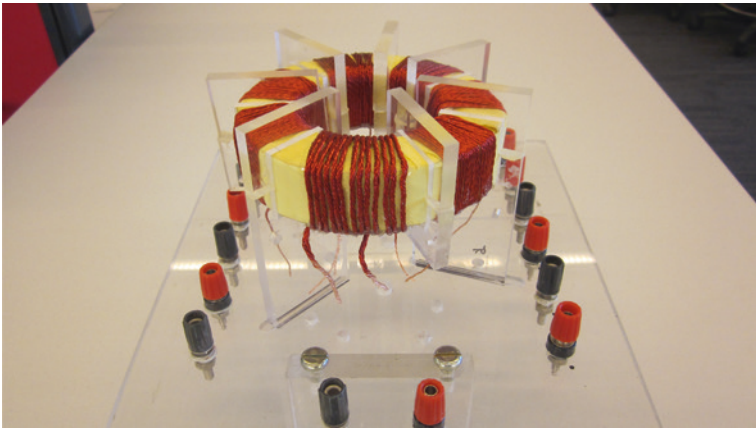
Fig. 4.30 Photograph of high-frequency magnetic link with Metglas alloy 2605S3A core
