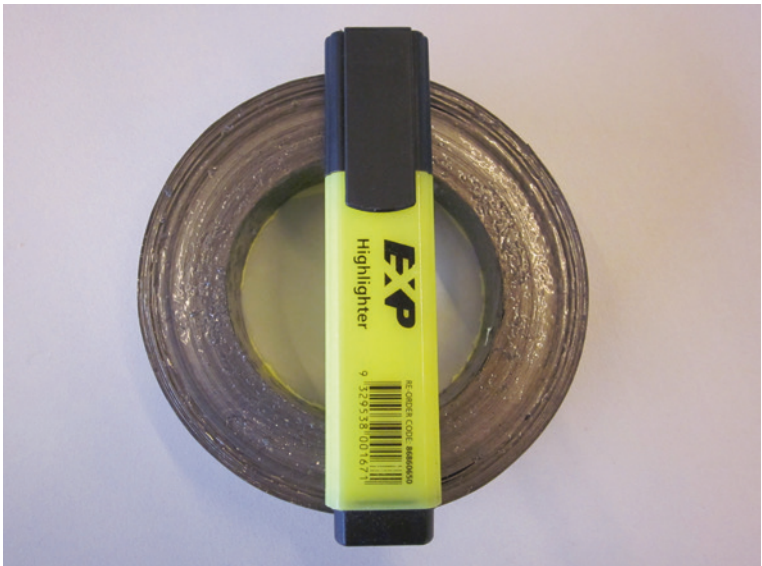
Fig. 4.28 Photograph of the transformer core with Metglas alloy 2605SA1 ribbon of 30 \mu\text{m} thickness and 25 mm of width
