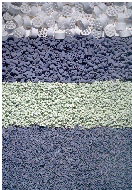
Figure 6.3. Typical hydrotreating catalysts. Reproduced with permission from Haldor Topsøe A/S.
