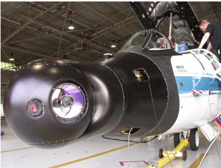
Fig. 9 WB-57F aircraft with WAVES nose cone. The large mirror is about the size of the 30 cm aperture of the ATOMMS instrument. (Figure provided courtesy of M. Ross)
