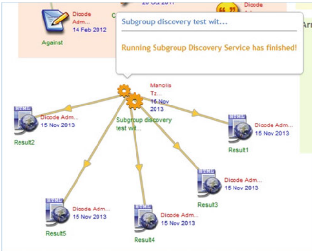
Fig. 6.2 A service item on the collaboration workspace has finished the execution of the subgroup discovery service. The outcomes of the execution are automatically uploaded and related in the workspace (items “Result1”–“Result5”)
