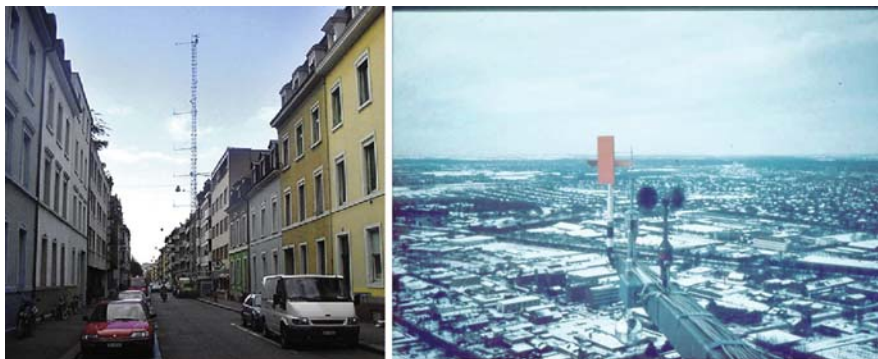
Fig. 12.2 (a) Mast in the BUBBLE experiment (Rotach et al., 2004) where measurements represent the roughness sub-layer. (b) Copenhagen experiment (Gryning and Lyck, 1984) where the measurements were performed above the roughness sub-layer
