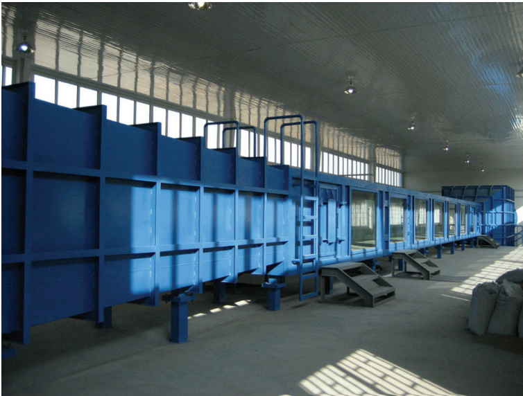
Fig. 2.7. Low-speed blow down wind tunnel (Multi-function environmental wind tunnel of Lanzhou University), which contains four sections: the power part, the rectifier part, the experimental part and the proliferation part. The total length of the wind tunnel is 85 m, the experimental section is up to 20 m, the cross-sectional area is about 1.3 m (width) \times 1.45 m (height), wind velocity is adjustable from 4 \text{ m}\cdot\text{s}^{-1} to 40 \text{ m}\cdot\text{s}^{-1}
