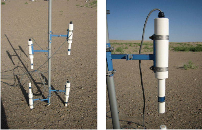
Fig. 2.6. The piezoelectric kinetic sensor for impact events measurement, with a frequency of 1 Hz which can be used to measure sand saltation activity (placed in Minqin, China by the author et al.)
