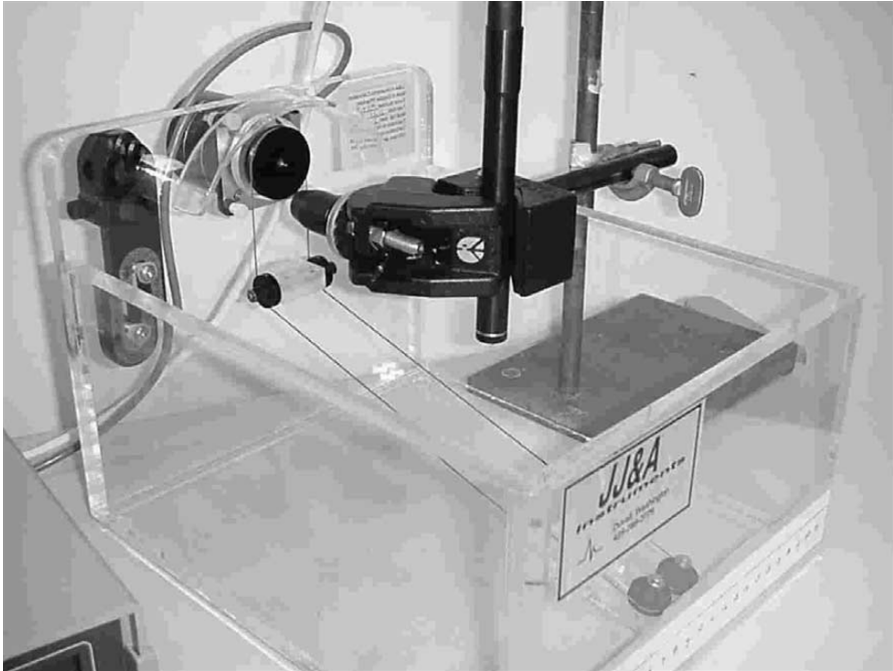
Figure 2. String phantom for assessment of Doppler velocity measurement (JJ&A Instr.).
