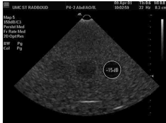
Figure 5. Echographic image obtained from scattering “lesions” and measurement disc inserted in one of them.
